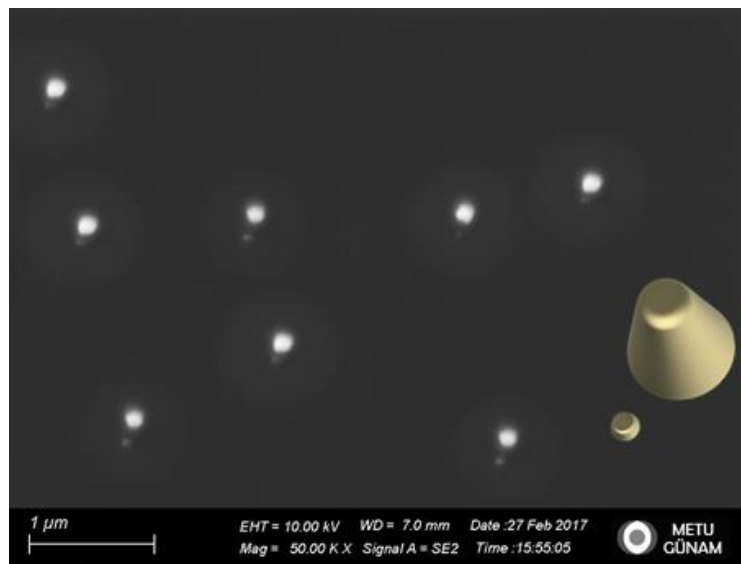
Figure 3.8. SEM image of highly asymmetric Ag dimers fabricated by HMCL by utilization of hole shrinkage
