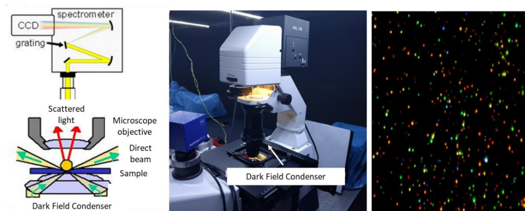
Figure 3.21. Left: schematic of dark field spectroscopy. Mid: The inverted microscope setup used in measurements. Right: A dark field image of a surface with different plasmonic resonances.
