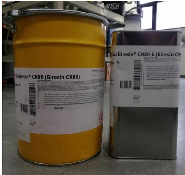
Figure 3.1. CR80 - CH80-6 epoxy resin system used in the study.
