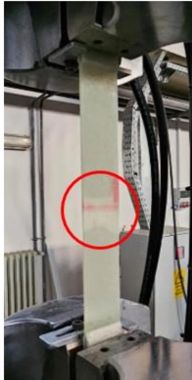
Figure 3.26. Delamination identification during the test.
