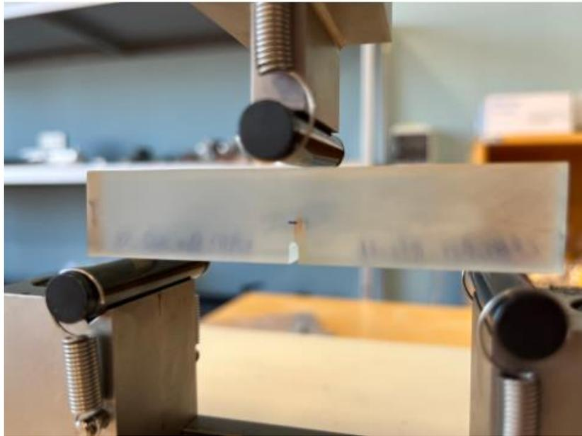
Figure 3.16. Fracture toughness specimen inside testing apparatus.
