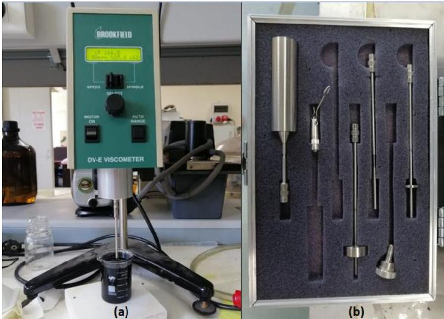
Figure 3.14. (a) Viscometer used in this study and (b) its spindles.
