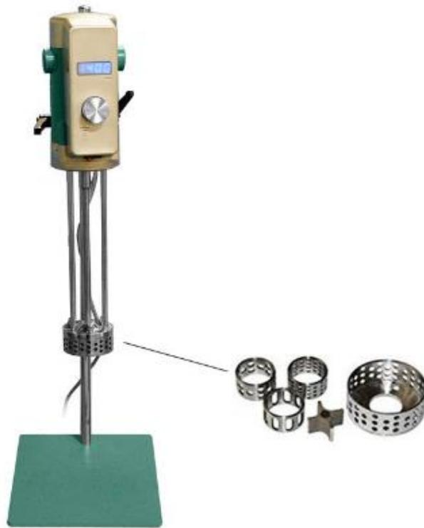
Figure 2.10. High-Shear Mixer.
