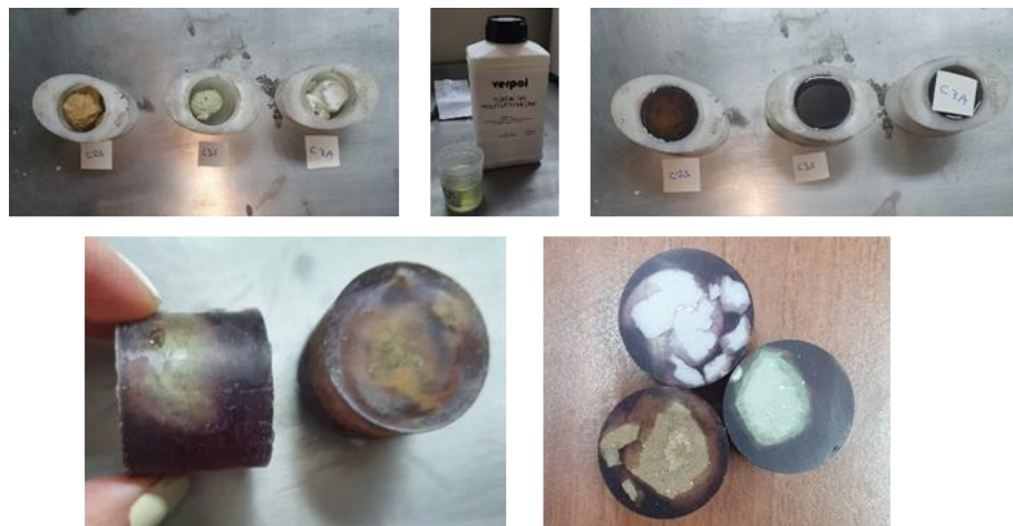
Figure 3-12 Steps for molding cement compound for polish sectioning for HIS
