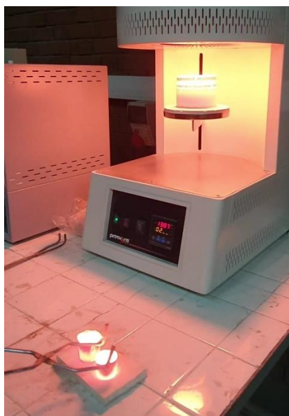
Figure 3-9 Hot crucible while removed from the furnace
