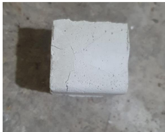
Figure 4-17 Cracks generation after 4 days of hydration in C_3A sample
