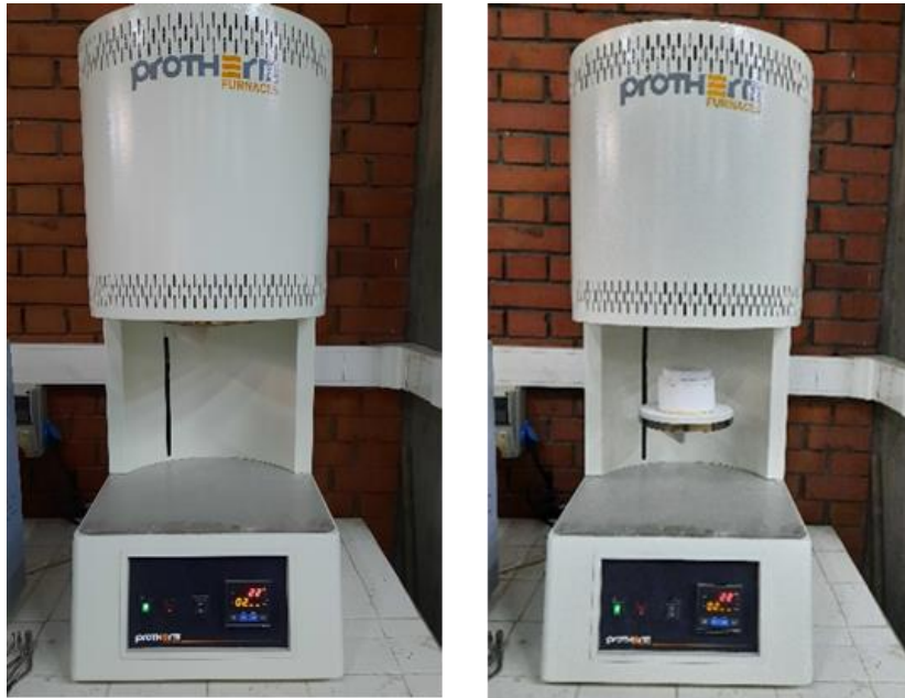
Figure 3-8 Protherm ELV MOS 160 furnace showing the elevated specimen holding platform on the right
