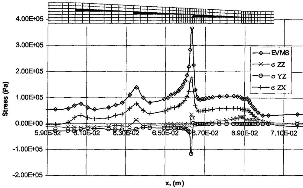
Figure 3.43: Equivalent Von Mises Stress and Interlaminar Stresses in Upper Interply Resin Layer Over the Tapered Region
