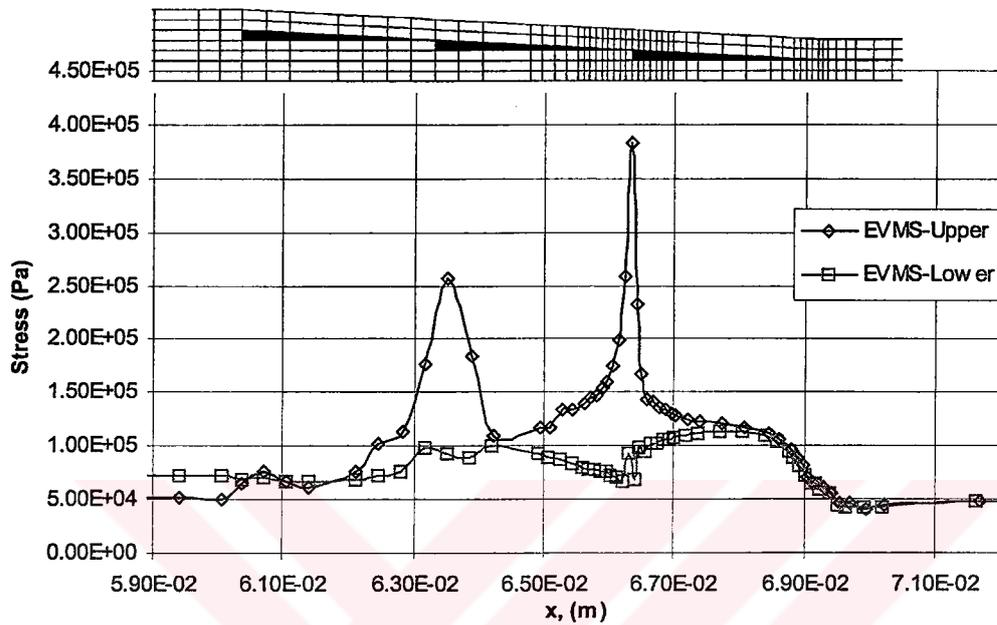
**Figure 3.22:** Equivalent von Mises Stresses in Upper and Lower Interply Resin Layers Over the Tapered Region
