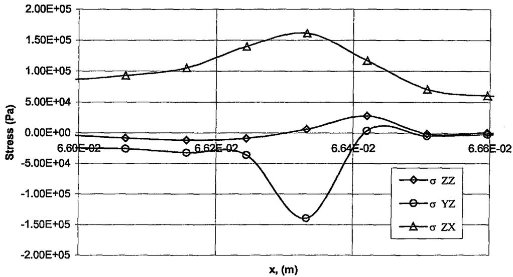
**Figure 3.31:** Interlaminar Stresses at the Predicted Delamination Onset Site
