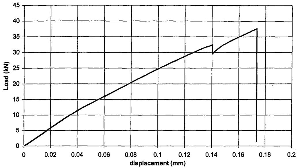
**Figure 4.17: Delamination of Specimen TL3-1**
