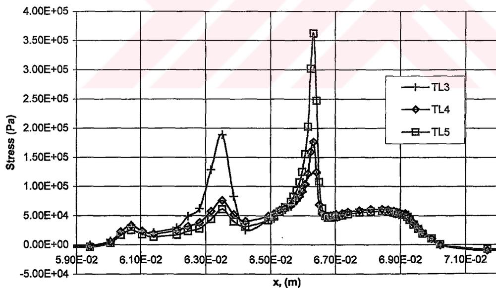
**Figure 5.2:** Interlaminar Shear Stresses in the Upper Interply Resin Region for TL3, TL4, and TL5
