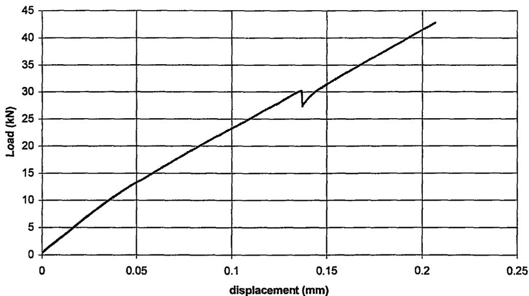
**Figure 4.19: Delamination of Specimen TL5-4**
