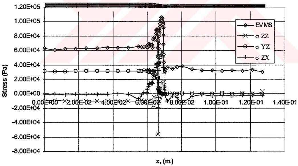
**Figure 3.42:** Equivalent Von Mises Stress and Interlaminar Stresses in Lower Interply Resin Layer Over the Entire Model
