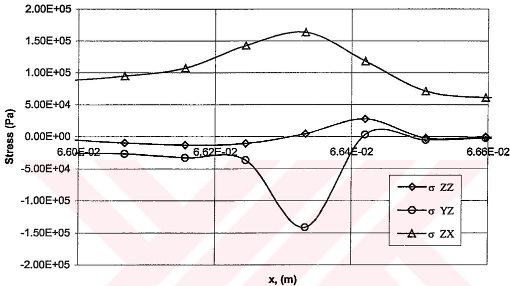
Figure 3.24: Interlaminar Stresses at the Predicted Delamination Onset Site
