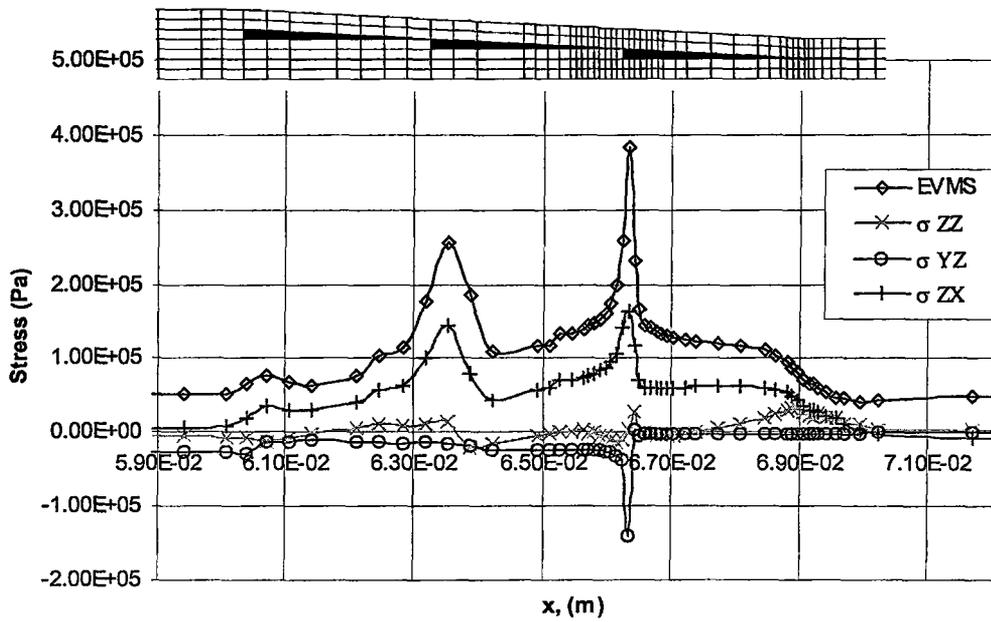
**Figure 3.20:** Equivalent von Mises Stress and Interlaminar Stresses in Upper Interply Resin Layer Over the Tapered Region
