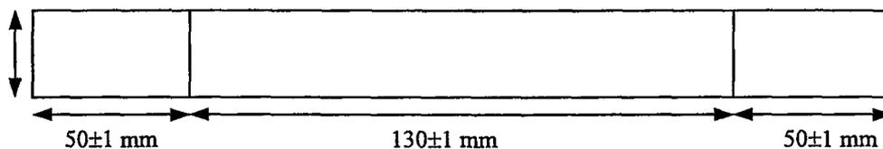
**Figure 4.2:** In-plane Shear Specimen Geometry
