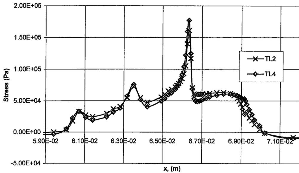
**Figure 5.4:** Interlaminar Shear Stresses in the Upper Interply Resin Region for TL2 and TL4
