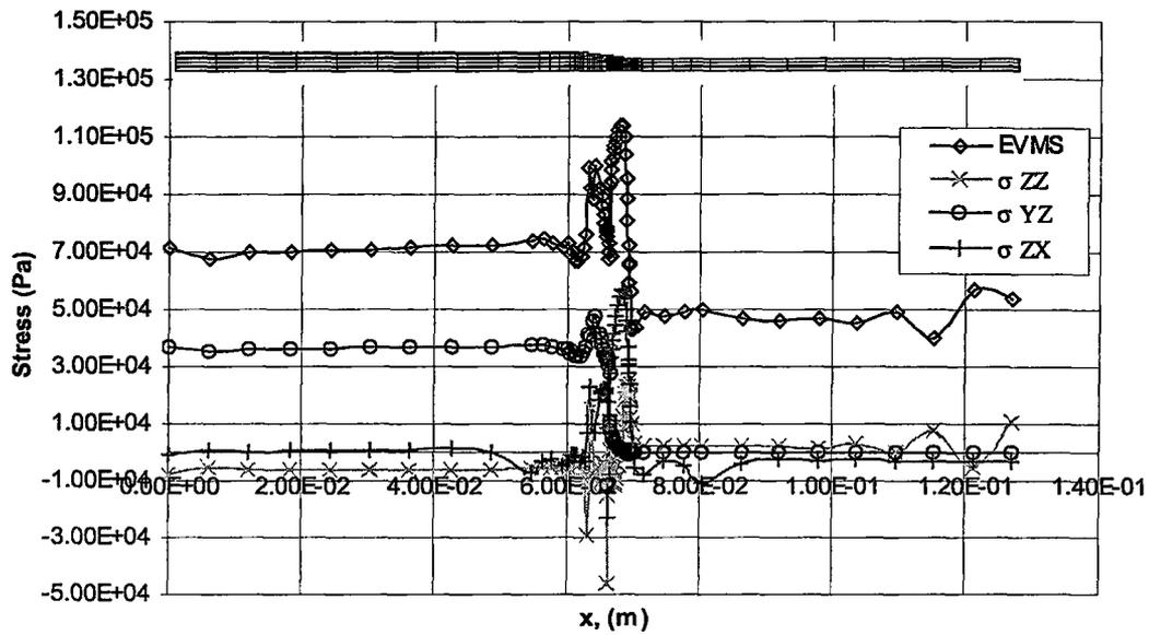
**Figure 3.19:** Equivalent von Mises Stress and Interlaminar Stresses in Lower Interply Resin Layer Over the Entire Model
