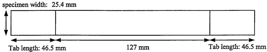
**Figure 4.13:** Specimen Dimensions for Flat Laminates
