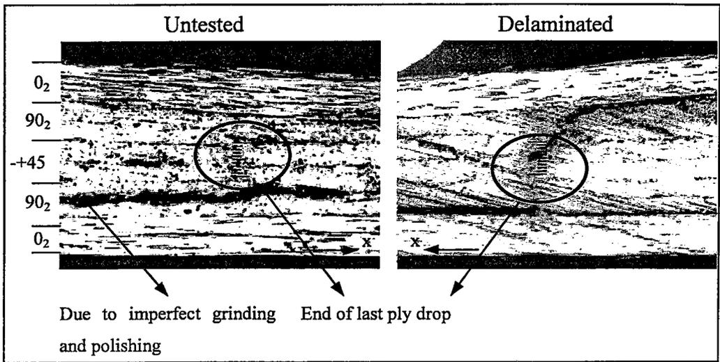
**Figure C.2:** Photomicrographs of configuration TL2
