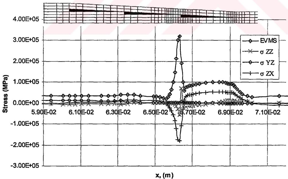
Figure 3.51: Equivalent von Mises Stress and Interlaminar Stresses in Lower Interply Resin Layer Over the Tapered Region
