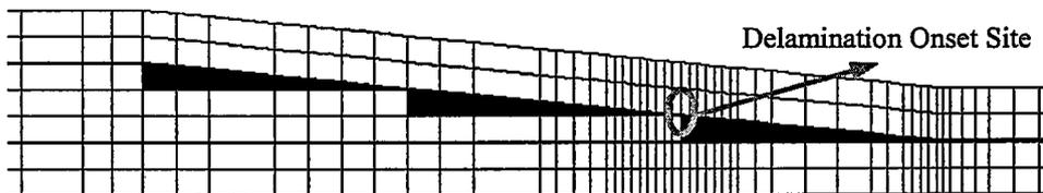
**Figure 3.30:** Predicted Delamination Onset Site for Configuration TL2
