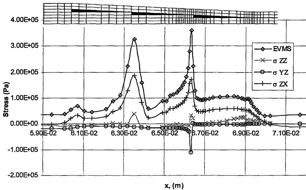
**Figure 3.36:** Equivalent von Mises Stress and Interlaminar Stresses in Upper Interply Resin Layer Over the Tapered Region
