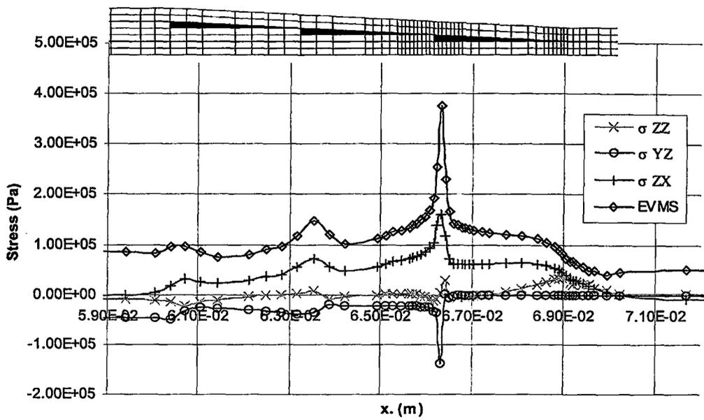
Figure 3.27: Equivalent von Mises Stress and Interlaminar Stresses in Upper Interply Resin Layer Over the Tapered Region
