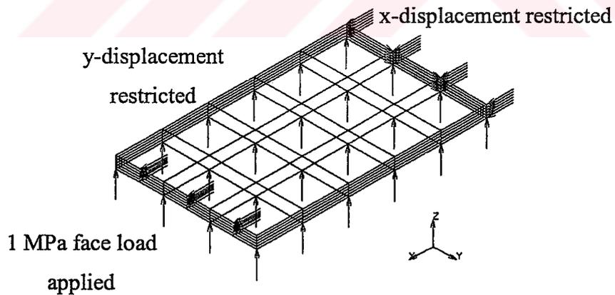
**Figure 3.3: Boundary Conditions Applied to the Basic Model**
