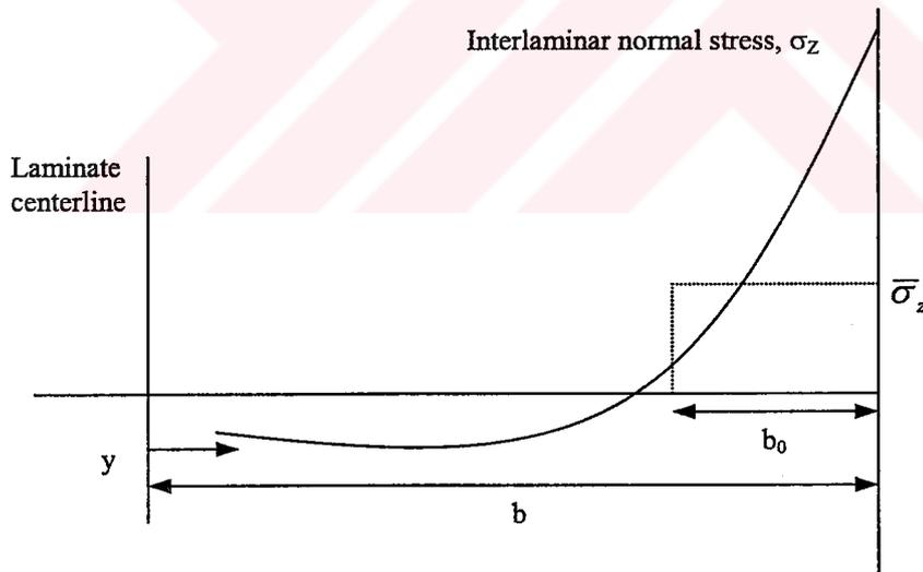
**Figure 2.1:** Graphical Interpretation of Average Interlaminar Normal Stress Near Free Edge According to the Kim-Soni Criterion.
