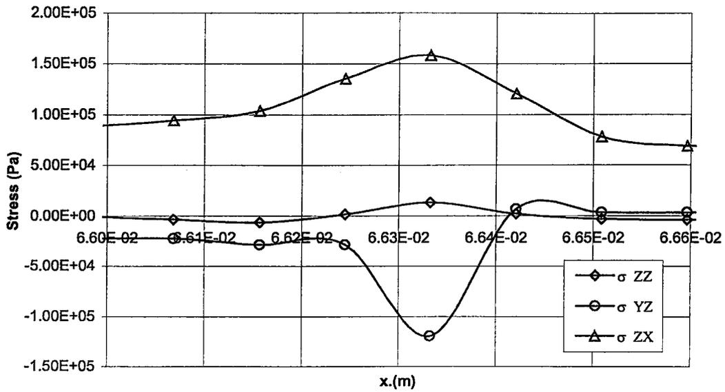
**Figure 3.32:** Interlaminar Stresses at the Predicted Delamination Onset Site for Configuration TL1-M
