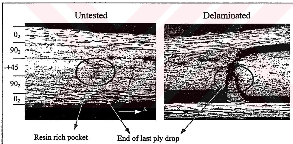
**Figure C.1:** Photomicrographs of configuration TL1
