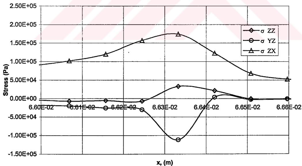
**Figure 3.40:** Interlaminar Stresses at the Predicted Delamination Onset Site
