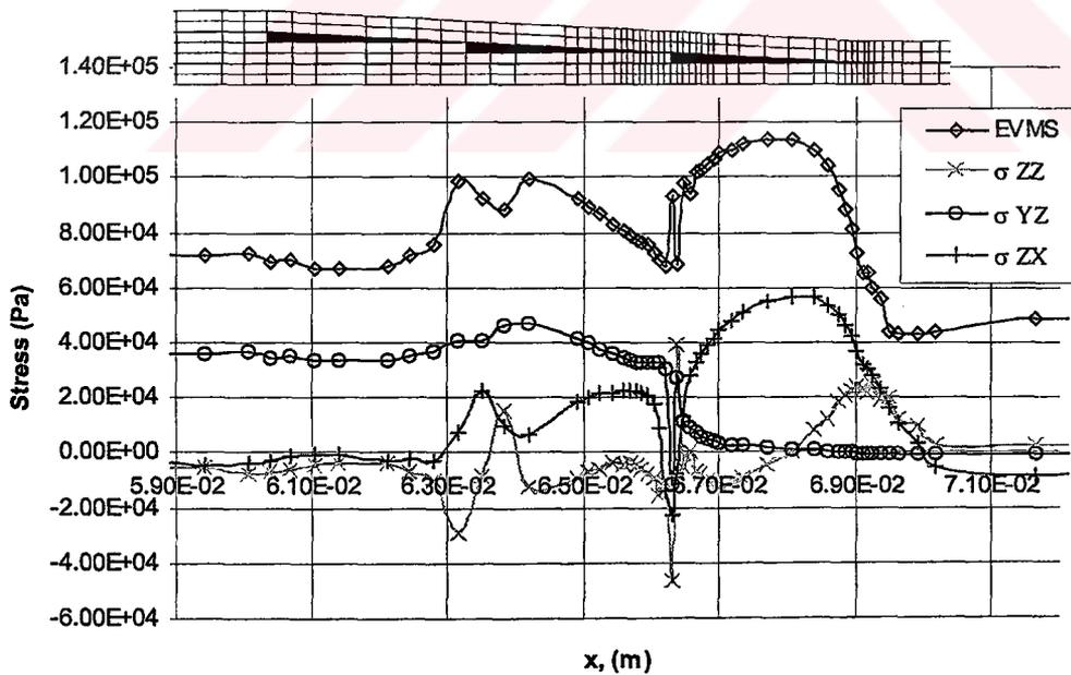
**Figure 3.21:** Equivalent von Mises Stress and Interlaminar Stresses in Lower Interply Resin Layer Over the Tapered Region
