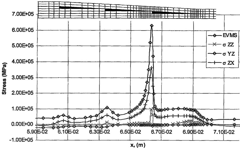
Figure 3.50: Equivalent von Mises Stress and Interlaminar Stresses in Upper Interply Resin Layer Over the Tapered Region
