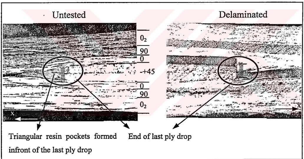
**Figure C.3:** Photomicrographs of configuration TL3
