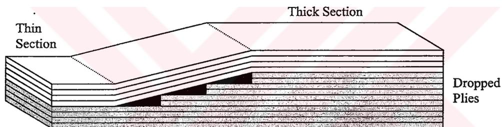
**Figure 1.2: Typical Tapered Laminate With Ply Drops**
