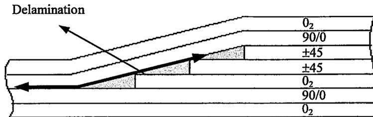
**Figure 4.20:** Delamination Path in TL5
