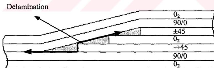
**Figure 4.18: Delamination Path in TL3**
