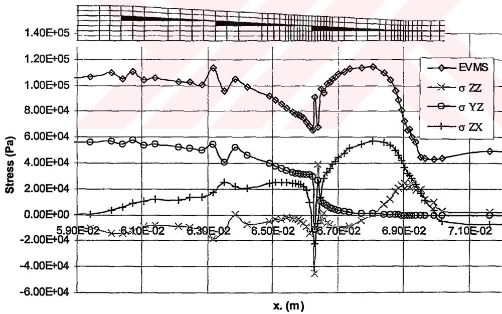
Figure 3.28: Equivalent von Mises Stress and Interlaminar Stresses in Lower Interply Resin Layer Over the Tapered Region
