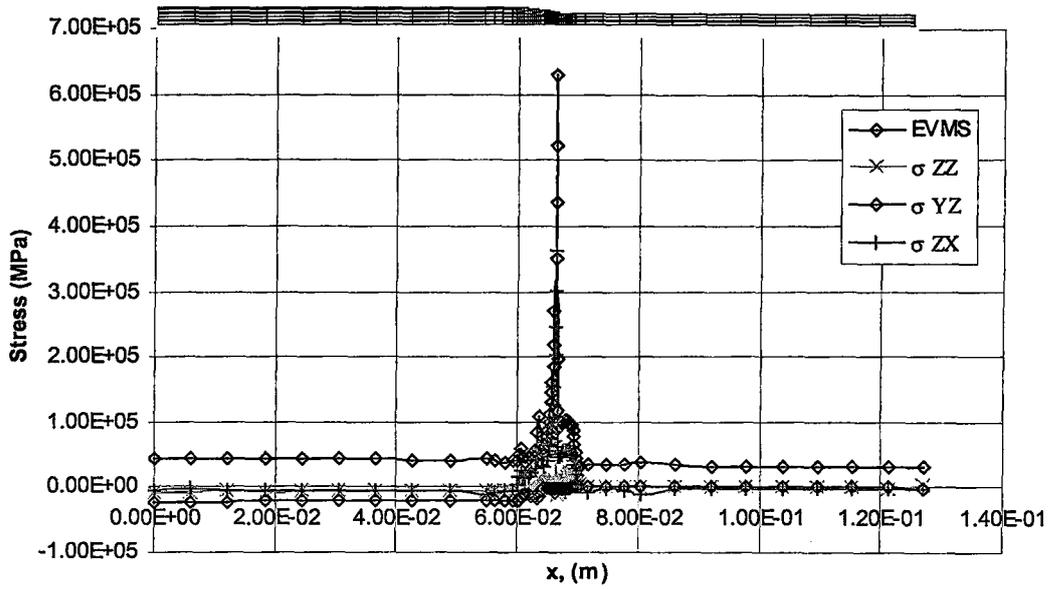
Figure 3.48: Equivalent Von Mises Stress and Interlaminar Stresses in Upper Interply Resin Layer Over the Entire Model
