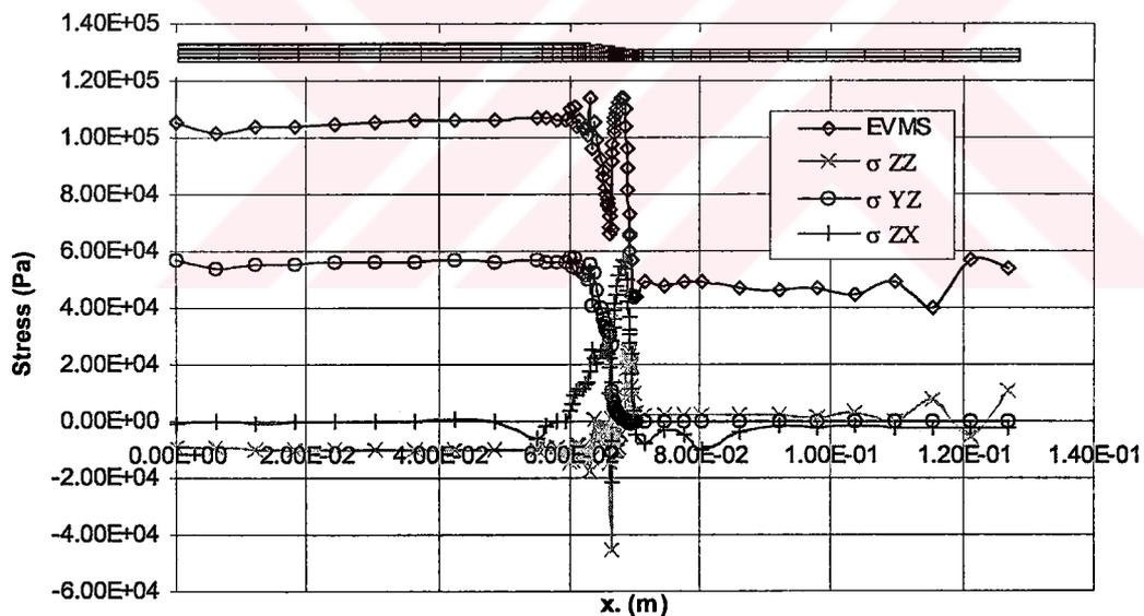
**Figure 3.26:** Equivalent von Mises Stress and Interlaminar Stresses in Lower Interply Resin Layer Over the Entire Model
