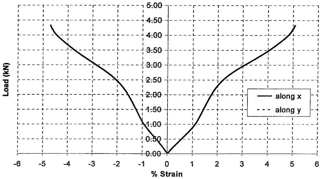
Figure 4.5: Load vs. % Strain Curve of the Test Specimen T $\pm 45^\circ$ -2
