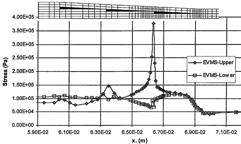
**Figure 3.29:** Equivalent von Mises Stresses in Upper and Lower Interply Resin Layers Over the Tapered Region
