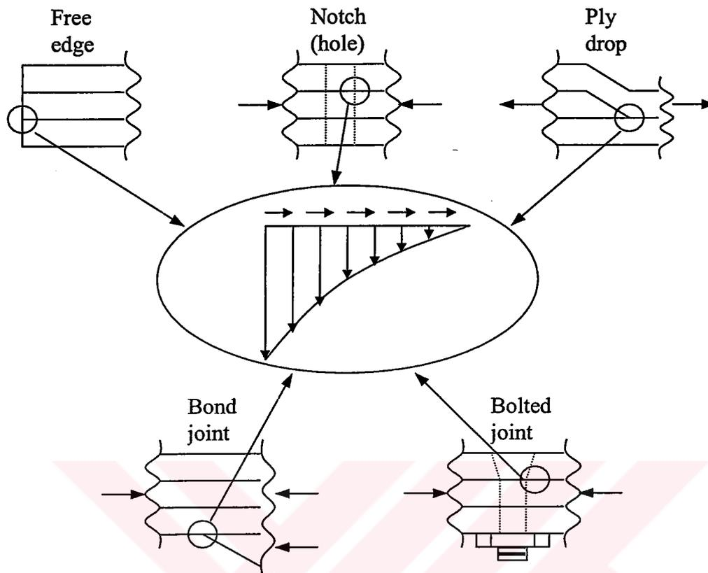
**Figure 1.3: Sources of Out-of-Plane Loads in Typical Aircraft Design**
