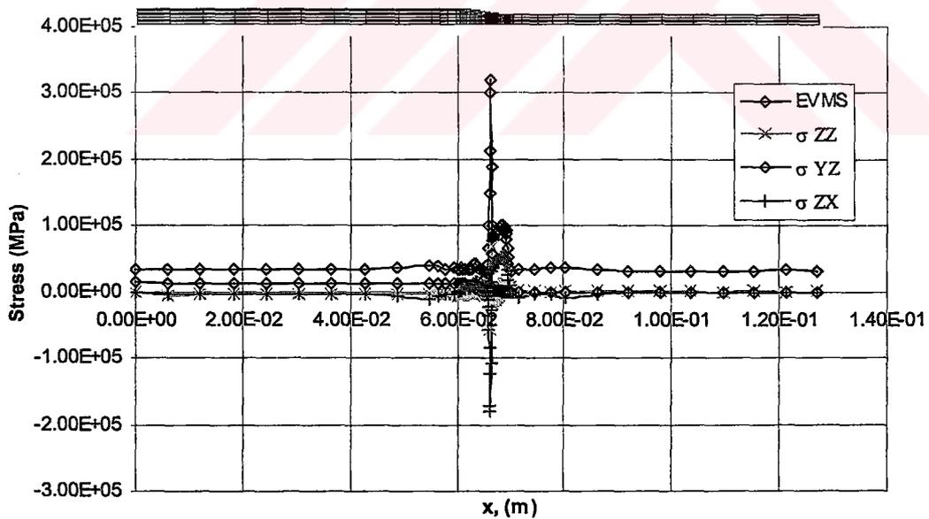
Figure 3.49: Equivalent von Mises Stress and Interlaminar Stresses in Lower Interply Resin Layer Over the Entire Model
