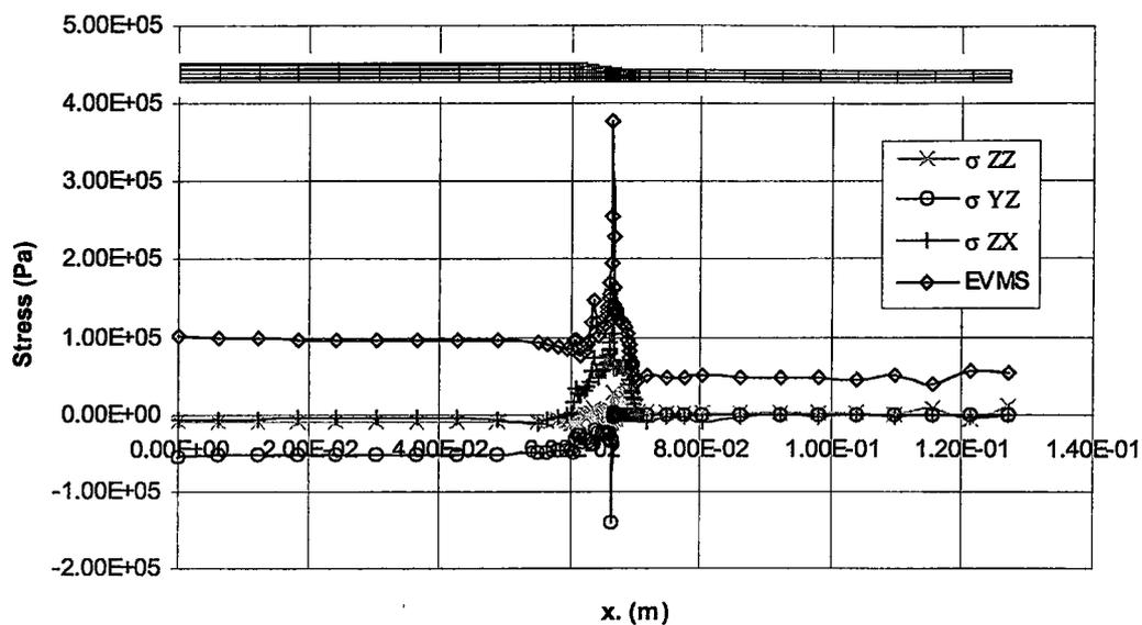
**Figure 3.25:** Equivalent von Mises Stress and Interlaminar Stresses in Upper Interply Resin Layer Over the Entire Model
