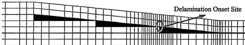
**Figure 3.39:** Predicted Delamination Onset Site for Configuration TL3
