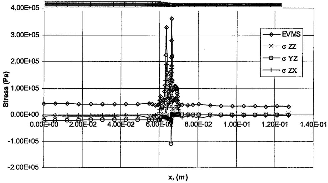
**Figure 3.34:** Equivalent von Mises Stress and Interlaminar Stresses in Upper Interply Resin Layer Over the Entire Model
