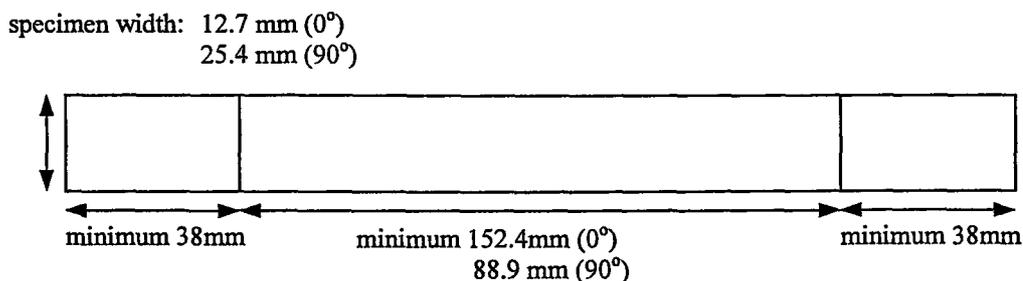
**Figure 4.1:** Tensile Specimen Geometry
