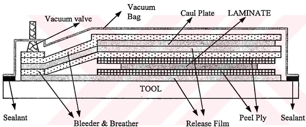
**Figure 4.7: Layup for Autoclave Curing**
