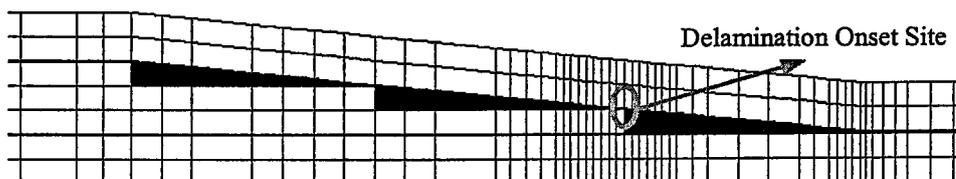
**Figure 3.23:** Predicted Delamination Onset Site for Configuration TL1
