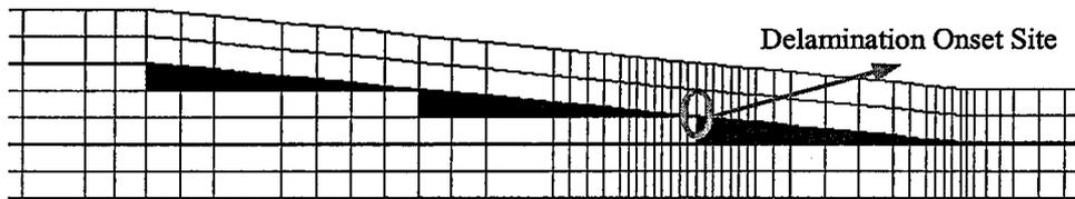
**Figure 3.46:** Predicted Delamination Onset Site for Configuration TL4
