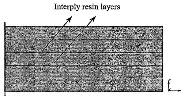
**Figure 3.4:** Interply Resin Layers in the Basic Model
