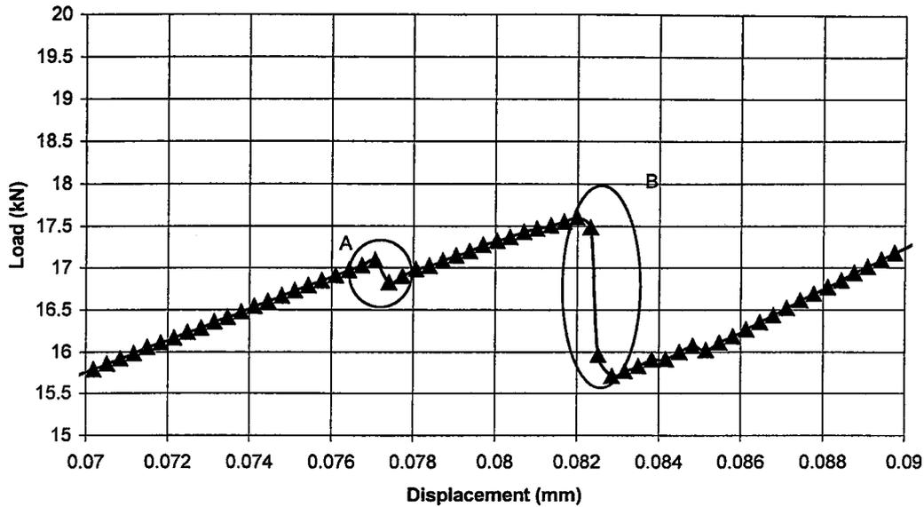
**Figure 4.15: Delamination Onset of Specimen TL1-3**
