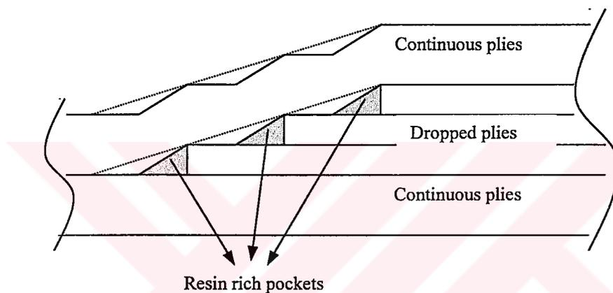
**Figure 4.8:** Shape Change Due to Curing
