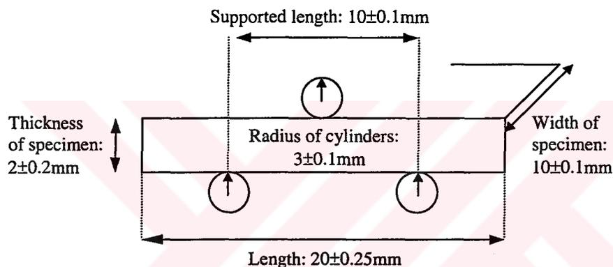
Figure 4.3: ILSS Test Specimen Geometry
