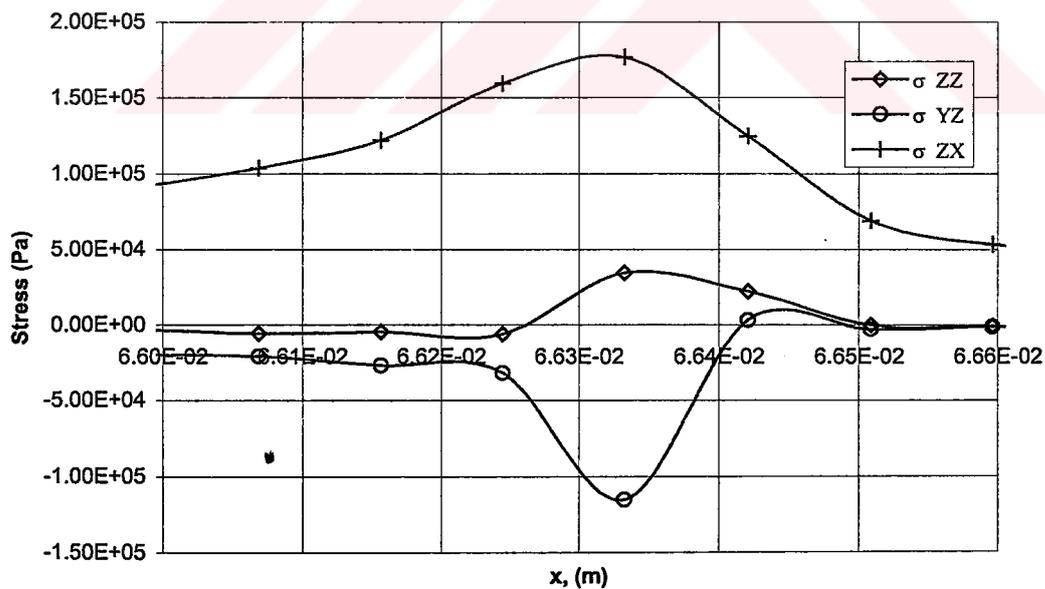
**Figure 3.47:** Interlaminar Stresses at the Predicted Delamination Onset Site
