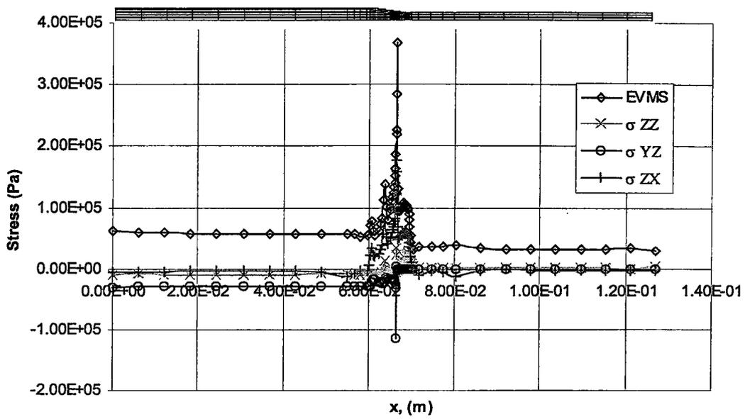
**Figure 3.41:** Equivalent Von Mises Stress and Interlaminar Stresses in Upper Interply Resin Layer Over the Entire Model
