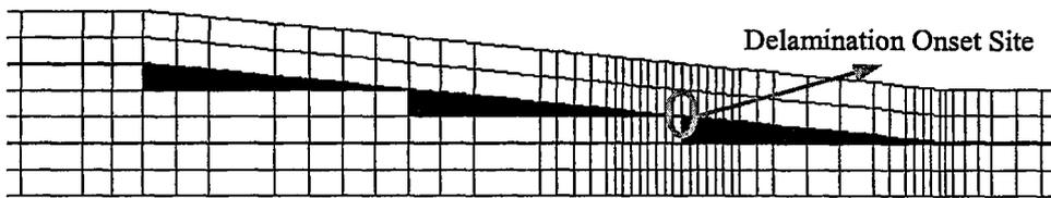
**Figure 3.53:** Predicted Delamination Onset Site for Configuration TL5
