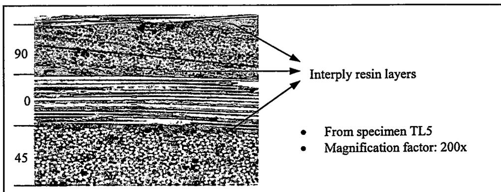
Figure C.6: Interply resin layers in configuration TL5
