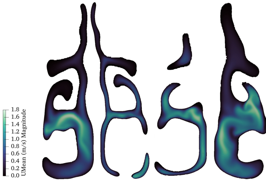
Figure 6.20. Velocity Magnitudes of the 11 th Slice for Pre-Surgery (Left) and Post-Surgery (Right): Restful State
