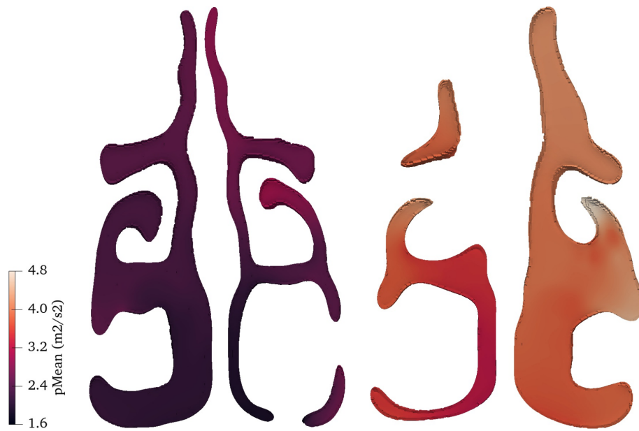
Figure 6.15. Pressures of the 11 th Slice for Pre-Surgery (Left) and Post-Surgery (Right): Restful State
