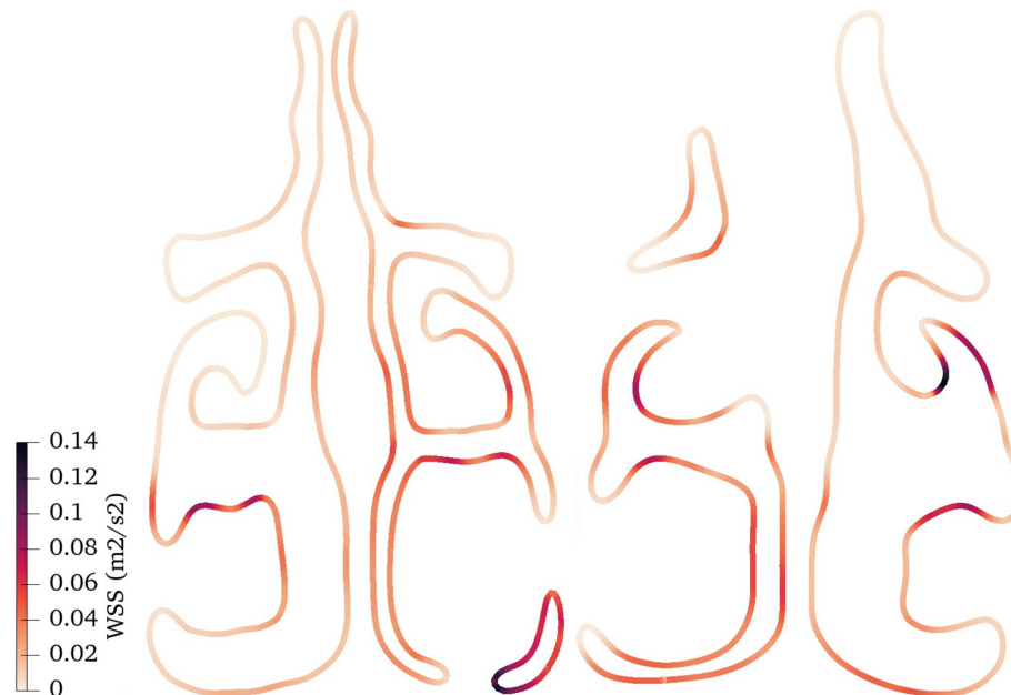
Figure 6.29. Wall Shear Stress Values for Pre-Surgery (Left) and Post-Surgery (Right): Restful Inhalation
