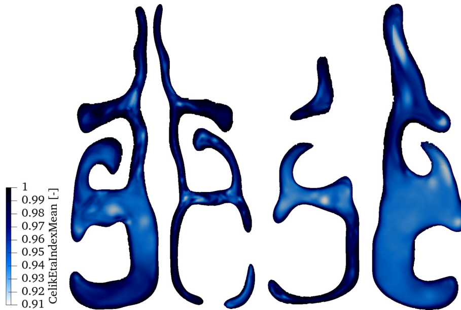
Figure 6.37. Kolmogorov Length Based Celik Index of the 11 th Slice for Pre-Surgery (Left) and Post-Surgery (Right): Quick State
