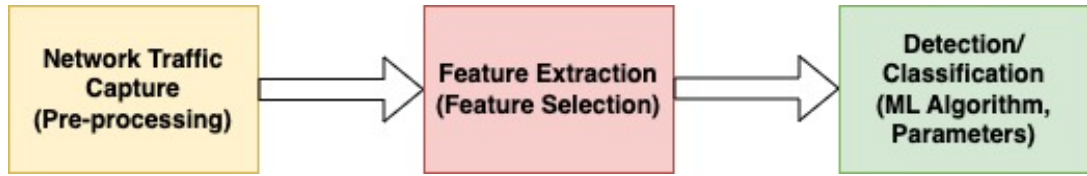
Figure 3: The pipeline of ML-based IDS
