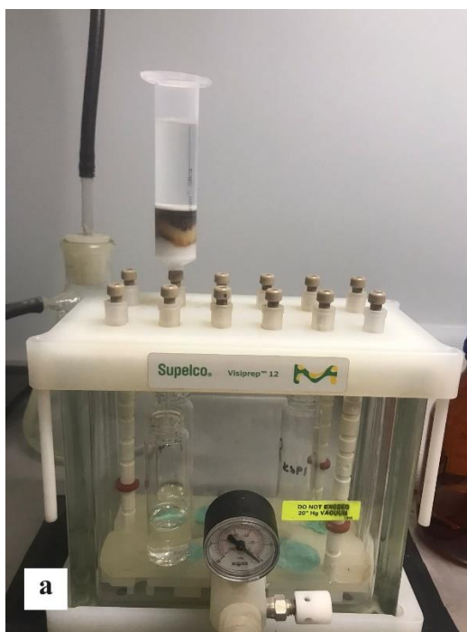
Figure 3.9. Toluene: n-heptane poured into SPE cartridge
