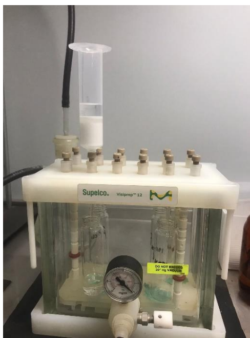
Figure 3.7. Process of pre-washing of SPE cartridge with 20 ml n-heptane
