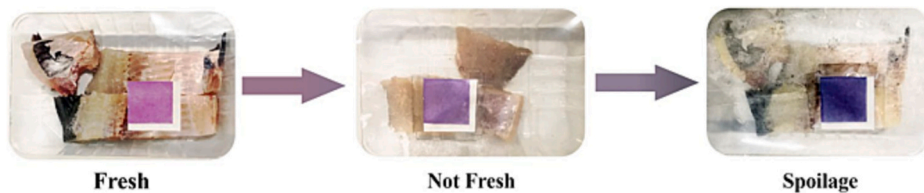
Fig. 7. (a) pH variations in grass carp stored at 25 °C within 24 h. (b) pH variability in grass carp stored at 4 °C over 7 days. (c) Changes in TVB-N values of grass carp kept at 25 °C within 24 h. (d) Shifts in TMA values of grass carp kept at 25 °C within 24 h. (e) Alterations in paper sensors' color while monitoring grass carp freshness within 24 h at 25 °C. Reprinted with permission from Springer [106]
