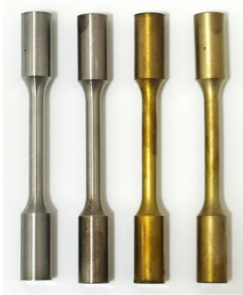
Figure 4.28 Tensile test specimens before testing, (a) as- received, (b) THPed (c) Nitrided + THPed, (d) Nitrided.
