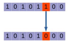
Figure 6. Example of bit inversion.
