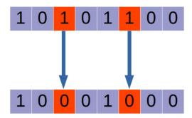
Figure 7. Example of mutation by exchange.
