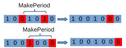
Figure 9. Example of the MakePeriod method.
