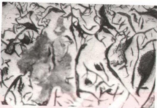
Figure 19. Sample 1.3. Etched with 2 % nital. X 200. Specimen 1.3 was poured 6 minutes after postinoculation.
