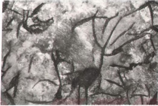
Figure 26. Sample 2.5. Etched with 2 % nital. X 200. Specimen 2.5 was postinoculated 10 minutes after Mg-inoculation.
