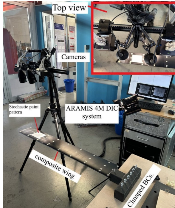
Figure 29. DIC test setup of composite wing.
