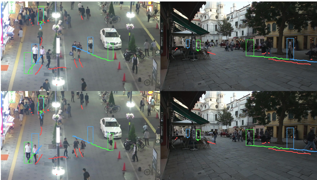
Figure 4.5: Results of visualizations of selected tracking examples. Blue lines indicates the query tracklet, red lines indicate the rejected matches, green line indicates the matched tracklet by the model.
