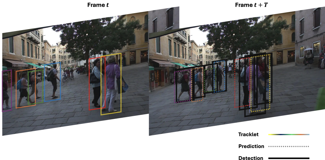
Figure 3.1: Kalman Filter based online tracking example. Colored bounding-boxes depict active tracks at frame t , dashed bounding-boxes represent the predicted positions of the tracklet at frame t + T , and black bounding boxes indicate the detections at frame t + T .
