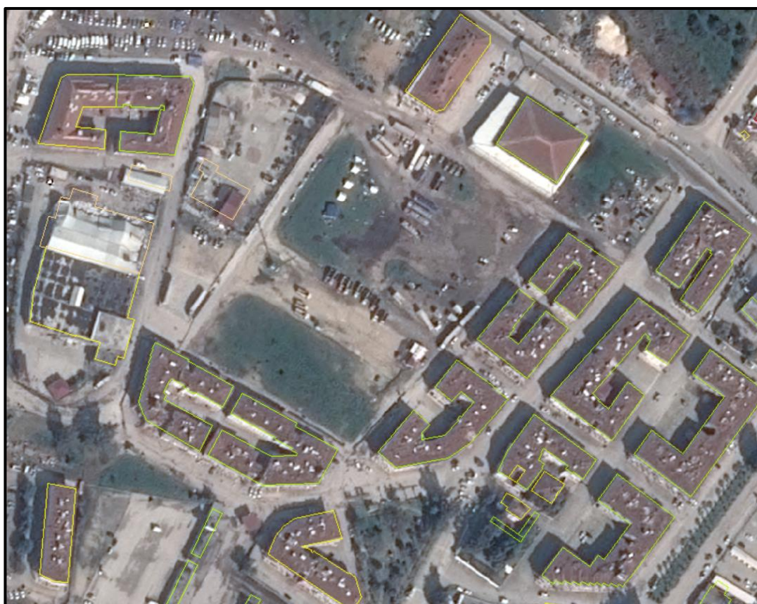
Figure 3.7. Post-edited vector data where the satellite image and vector data building footprints match.
