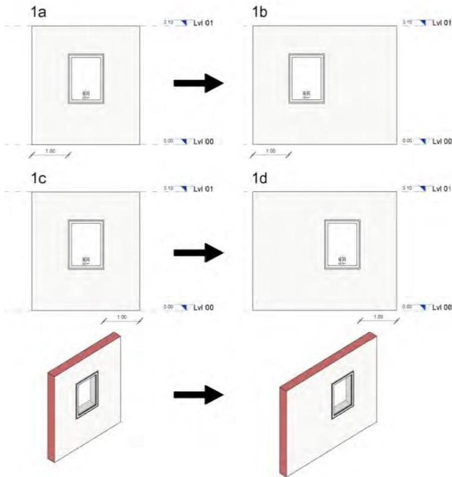
Figure 2.6. The relationship between the position of the window and the dimension change of the wall (Luciani et. al, 2012).
