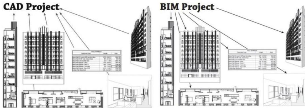
Figure 2.1. CAD-based and BIM-based workflows illustrated by Krygiel and Vandezande (2014).
