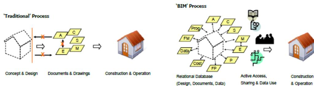
Figure 2.4. Traditional project (left) and BIM project (right) processes (Azhar et. al, 2012).
