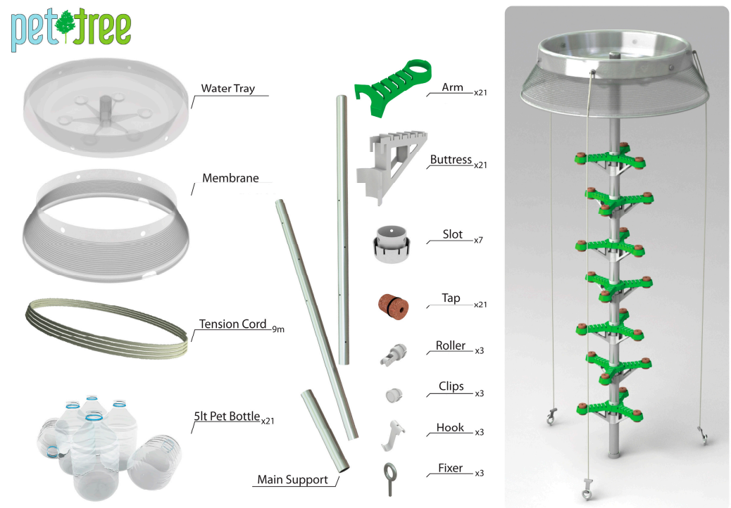
Figure 4. Recycled plastic injection molding parts of the system.
