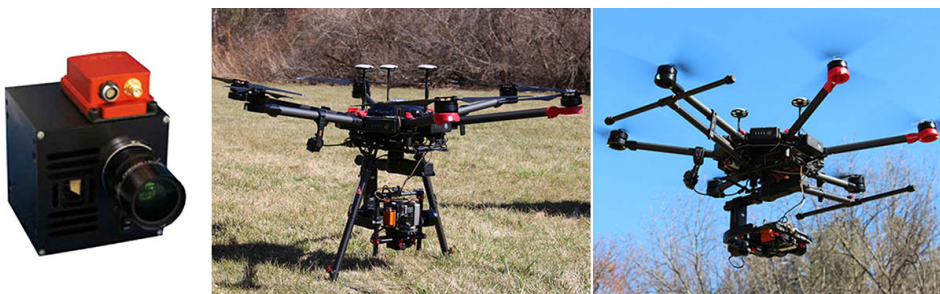
Figure 13: Nano-Hyperspec hyperspectral remote sensing system installed on DJI M600 Pro UAV.
