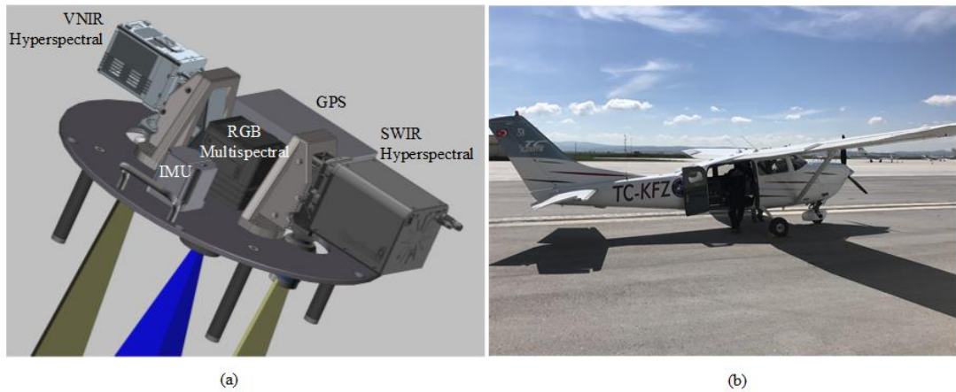
Figure 41: Multi-modal sensor configuration of the imaging system: a) sensors and auxiliary components, b) Cessna 206 manned airborne platform.
