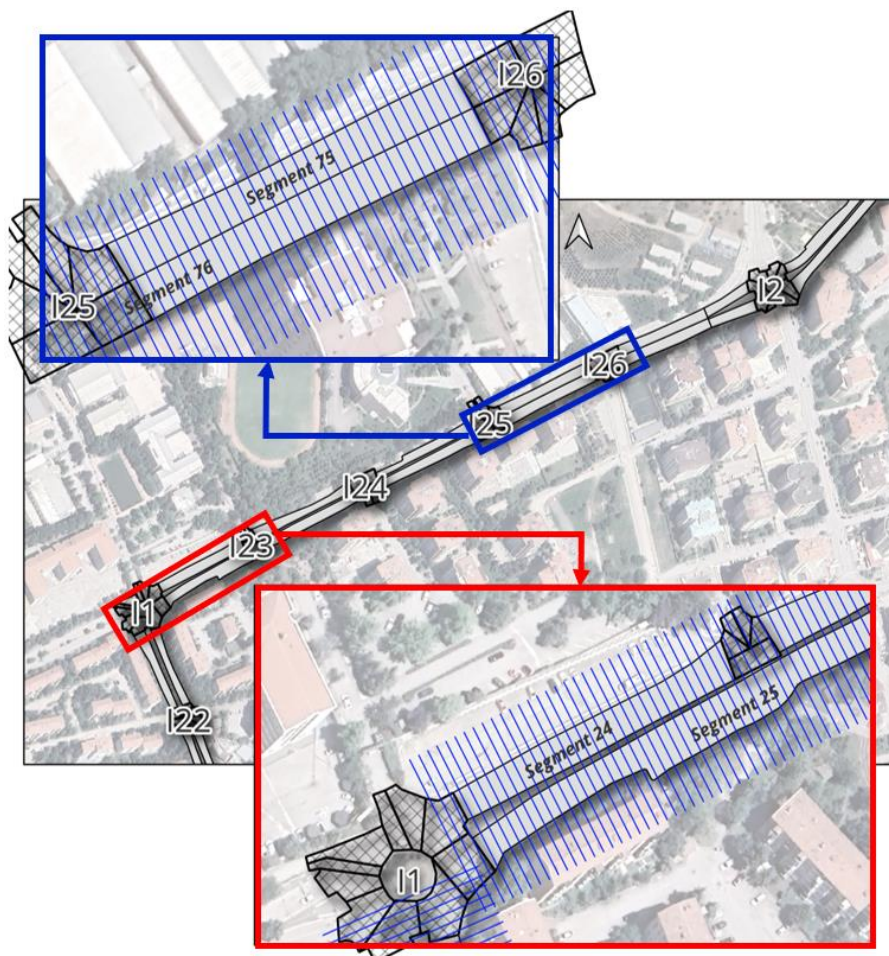
Figure 4.3 Segmentation and slicing between major intersections of I1, I23 and I25, I26.
