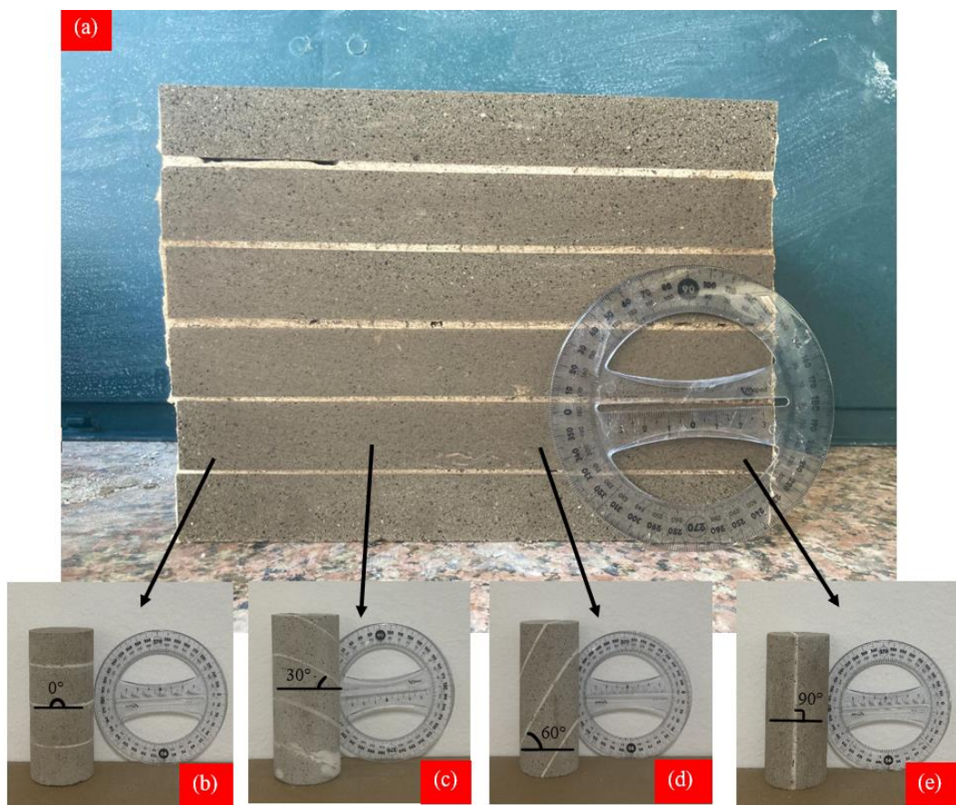
Figure 3.5. (a) bigger sized cubical block from which cylindrical samples were obtained, sample with fracture orientation of (b) 0°, (c) 30°, (d) 60°, (e) 90°
