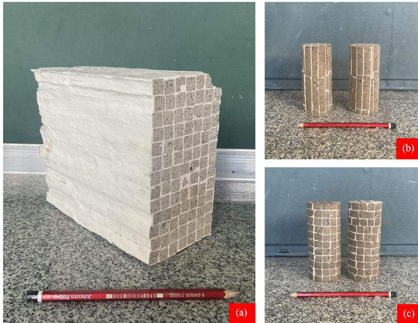
Figure 3.3. (a) bigger block constructed from the attachment of “layers” (b) Fine_BLL samples (c) Fine_BLS samples
