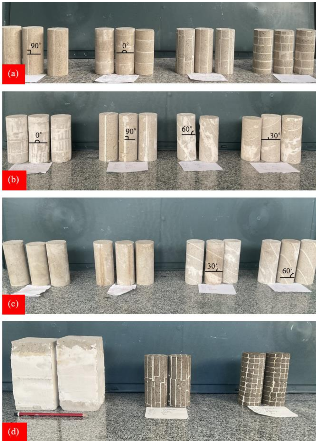
Figure 3.7. (a) samples LC_90, LC_0, Coarse_BLL, Coarse_BLS (from left to right) (b) samples HC_0, HC_90, HC_60, HC_30 (from left to right) (c) samples HC_C, LC_C, LC_30, LC_60 (from left to right) (d) samples Cubic, Fine_BLL, Fine_BLS (from left to right)
