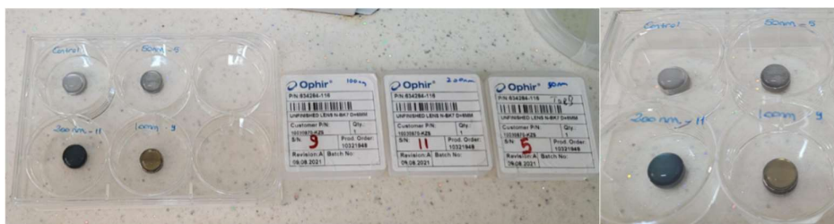
Figure 3.30. The samples on which 0.5 McFarland density bacteria added in six well plates
