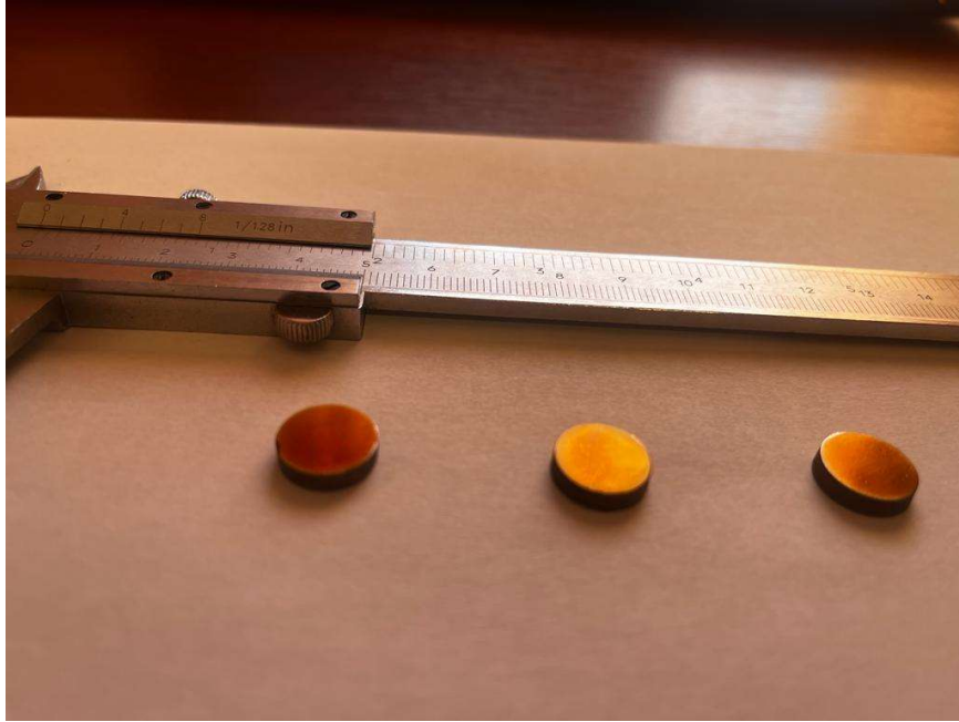
Figure 3.14. \text{TiO}_2 (25 nm) + DLC (150 nm) Coated 304 Steel Samples
