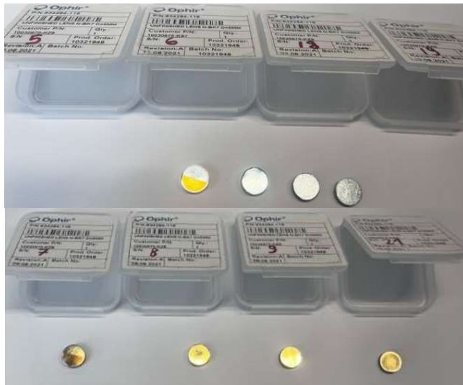
Figure 3.15. Samples Successfully Coated with 15 nm \text{TiO}_2 and Different Thicknesses (50/100/200 nm) of DLC
