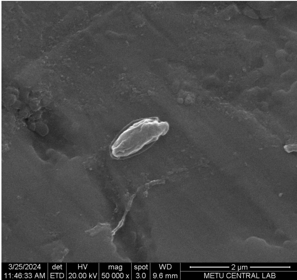
Figure 3.43. Mycobacterium chimaera on substrate which is coated with 100 nm DLC thin film.
