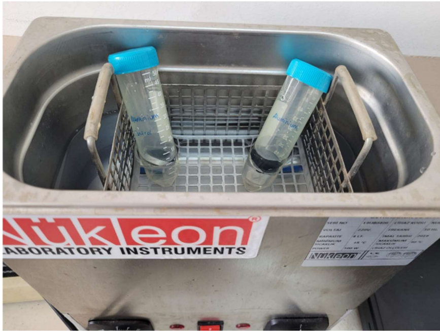
Figure 3.35. Removal process of bacteria form the surface by sonication
