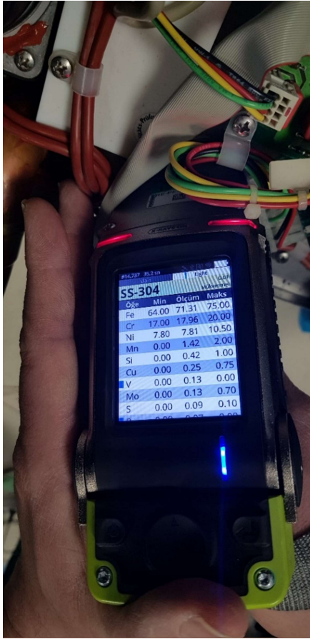
Figure 3.3. The handheld XRF Device Showing the Measurement Result
