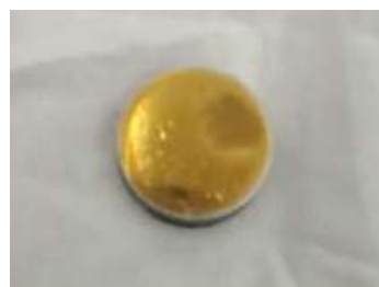
Figure 3.13. Sample #2 PVD Coating of \text{TiO}_2
