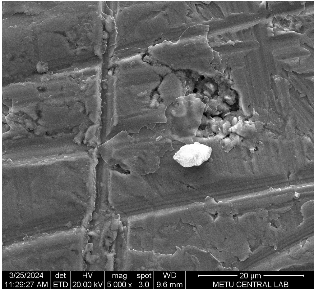
Figure D.47. FESEM image of Mycobacterium chimaera which is taken from the 200 nm DLC coated sample
