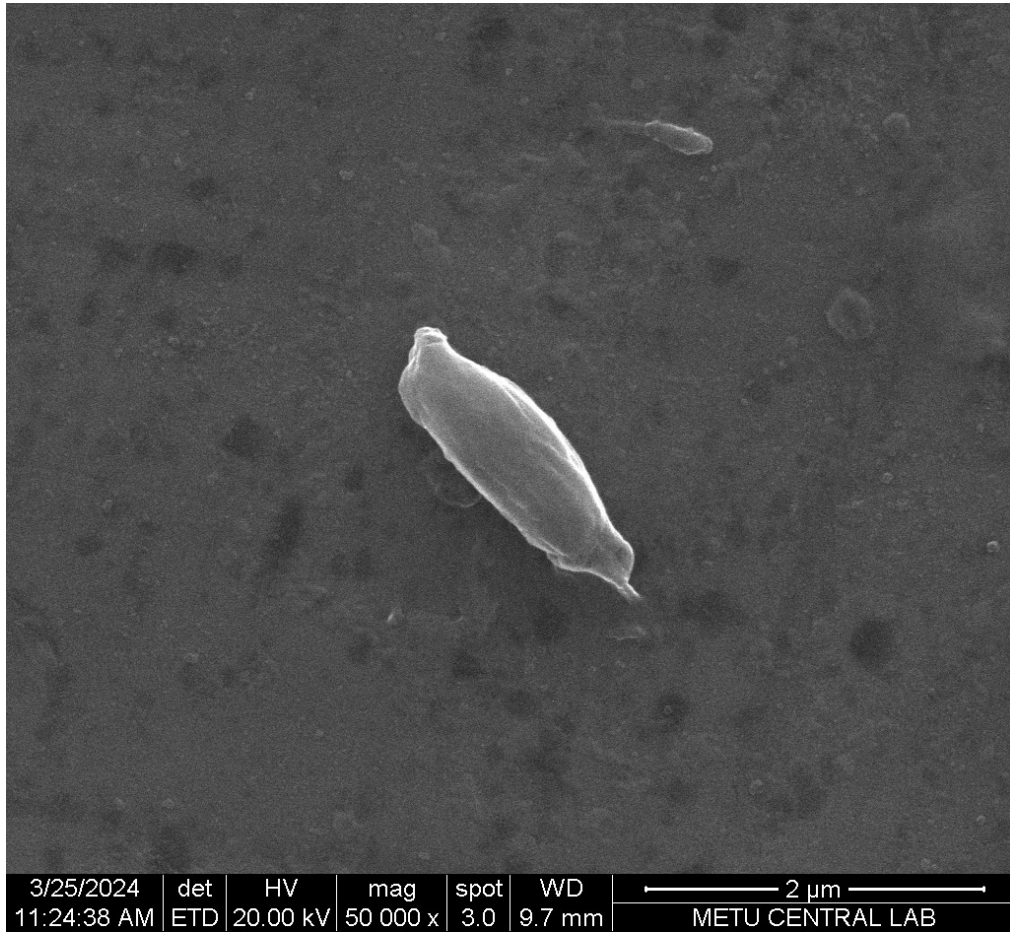
Figure D.37. FESEM image of Mycobacterium chimaera which is taken from the 100 nm DLC coated sample
