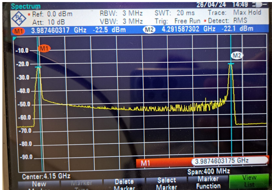
Figure 4.6: HMC391 VCO Band Measurement w/Oscilloscope
