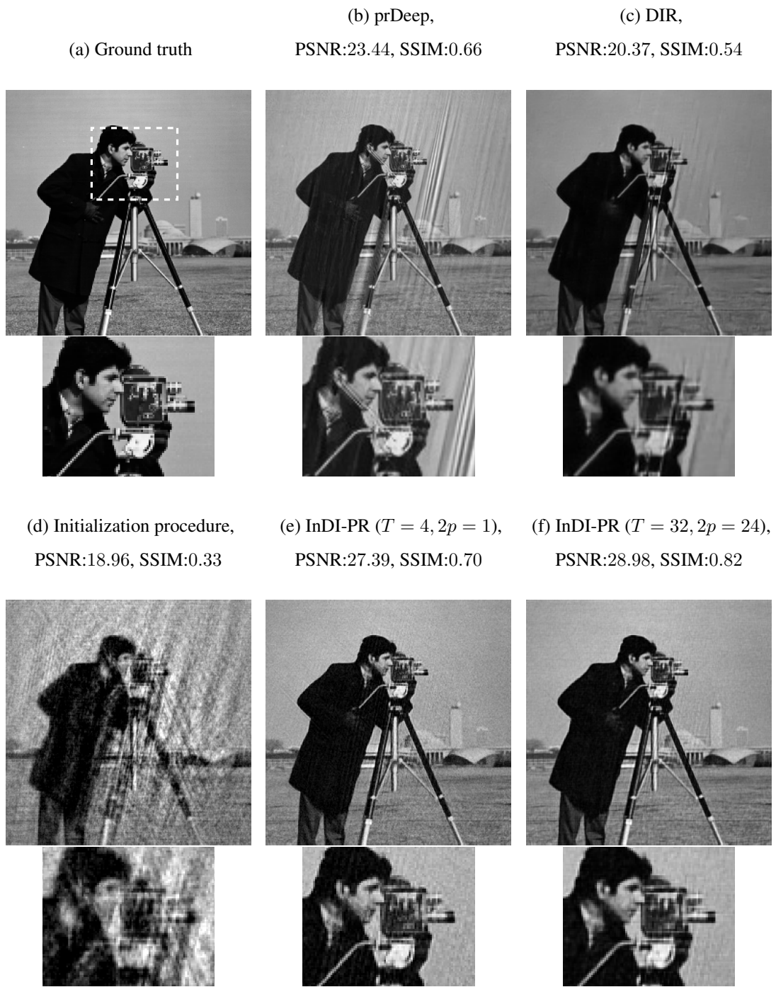
Figure 3.7: The outputs of various algorithms for the "Cameraman" test image subjected to \alpha = 3 noise (SNR=31.61dB).
