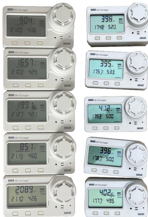
Figure 3.22 Before and after the calibration of HOBOWare data loggers. (2023)
