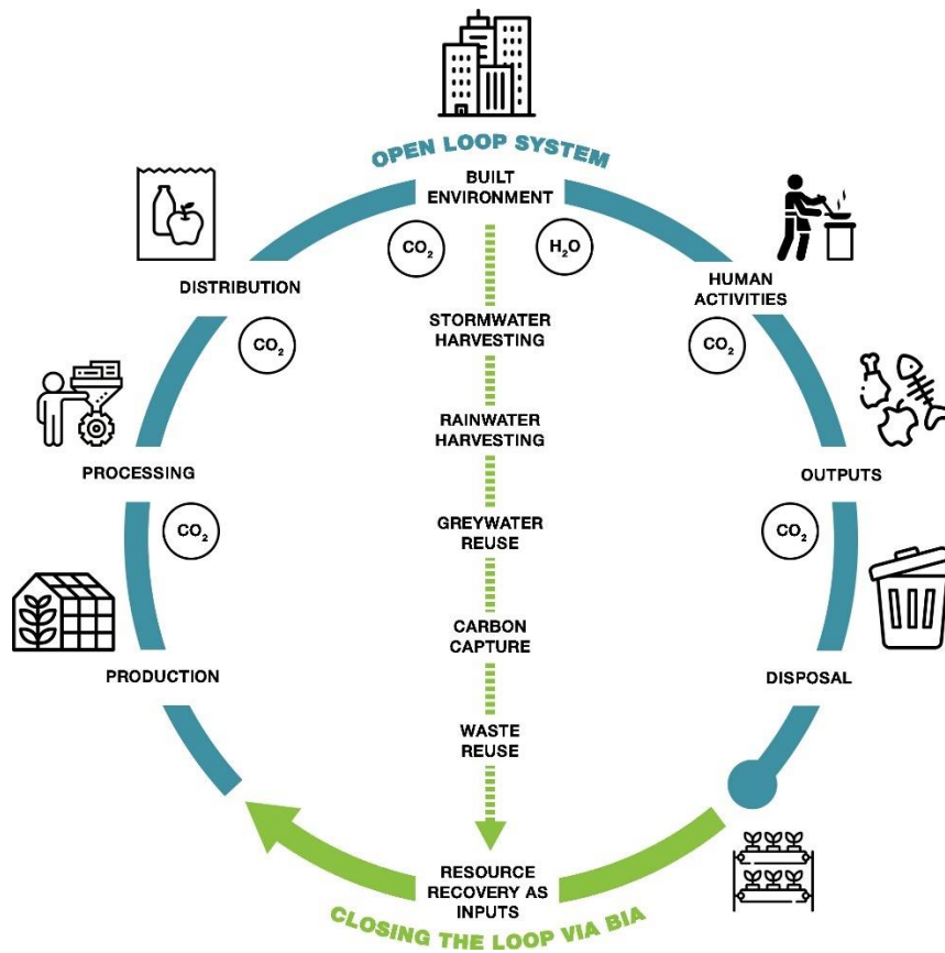
Figure 4.6 Closing the open loop systems via BIA systems in the proposed transformation scenario of the Sihhiye Multistorey Car Park.
