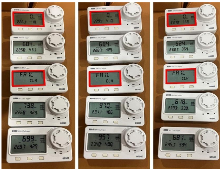
Figure 3.24 Errors of data loggers in the cafeteria as “altitude error” with 0 CO 2 ppm value and “Fail CLH error” for condensation risk. (16.05.2024)
