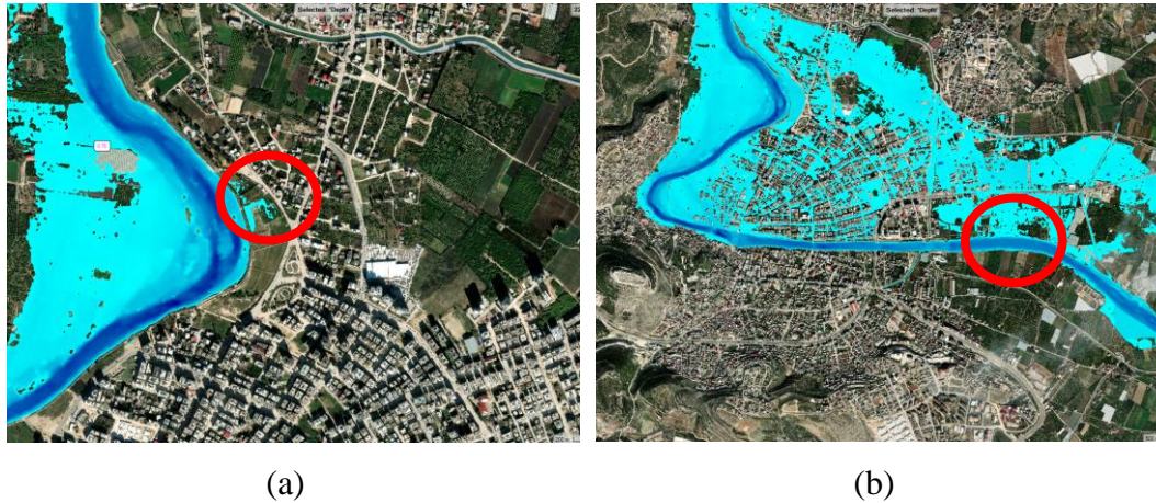
Figure 5.8. The combined 1D/2D hydraulic model results: (a) The location where flood water entered the center of Silifke (b) The location where flood water left the center of Silifke (Basemap source: ArcGIS World Imagery)
