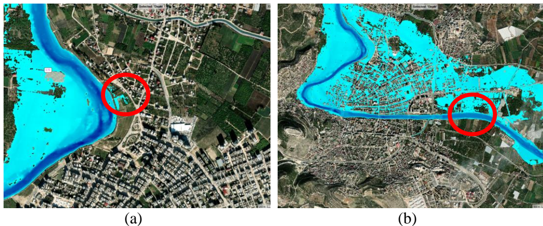
Figure 6. The combined 1D/2D coupled hydraulic model results: (a) The entering location of flood water (b) The leaving location of flood water (Basemap source: Esri, Maxar, Earthstar Geographics, and the GIS User Community)
