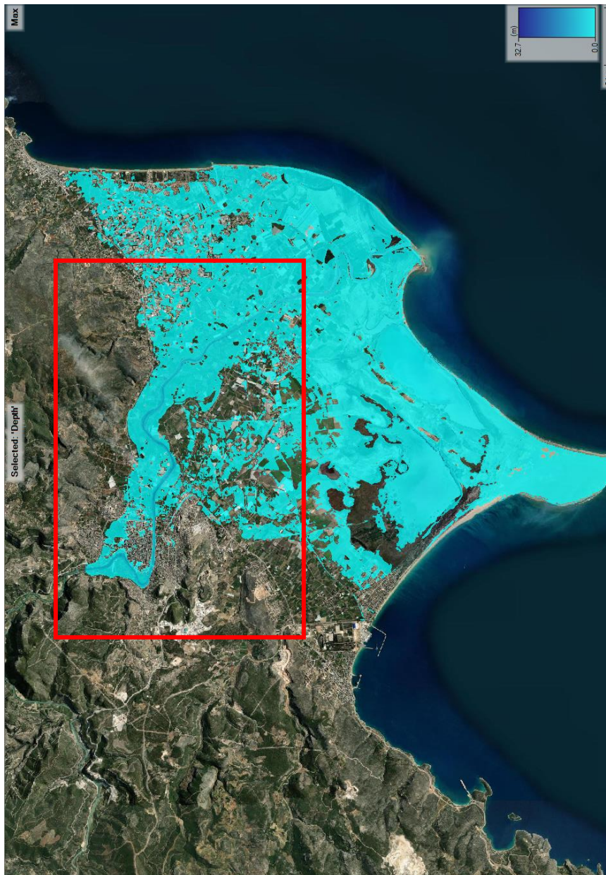
Figure 5.9. Q 500 flood inundation map under stationary conditions (S0) (Basemap source: ArcGIS World Imagery)
