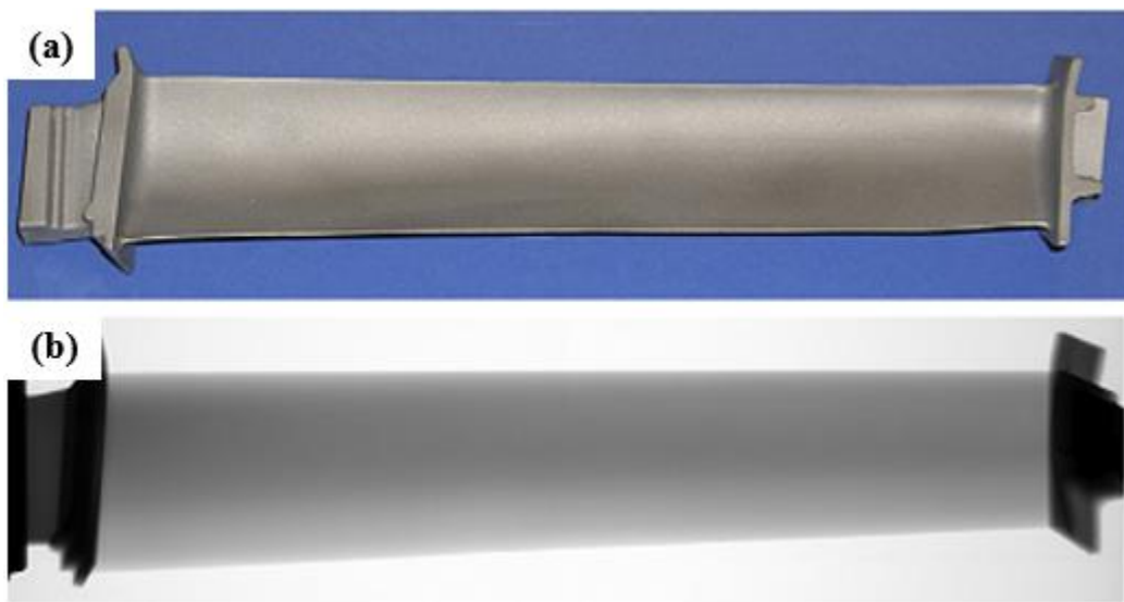
Figure 2.24: (a) An investing casted LPT blade and (b) its corresponding X-ray picture [149].
