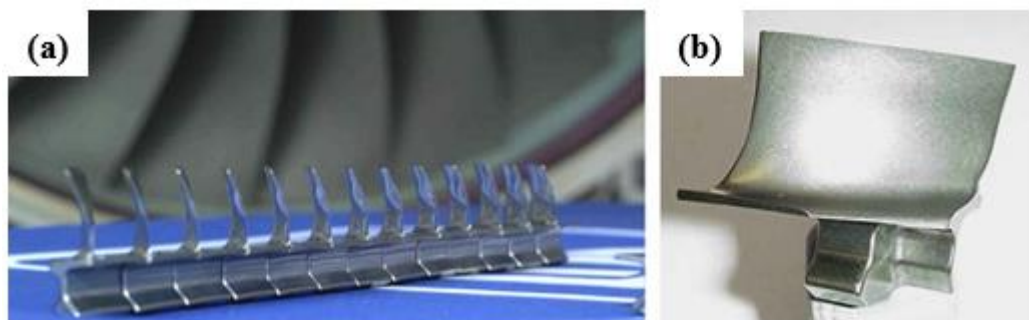
Figure 2.26: Compressor blades of Ti45Al8Nb0.5(B,C) produced using extrusion and forging process; (a) set of blades and (b) an individual blade [3].
