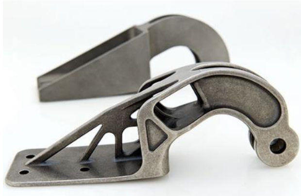
Figure 2.53: Airbus A320 engine attachment hinge; in the background: geometry produced with traditional methods, in the foreground: geometry produced with PBF-EB and topology optimization [219].
