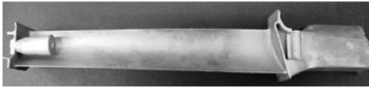
Figure 2.25: Centrifugally casted GEnx LPT blade [41].
