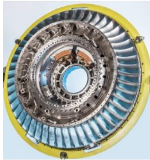
Figure 2.50: A front bearing housing produced by Rolls Royce [216].
