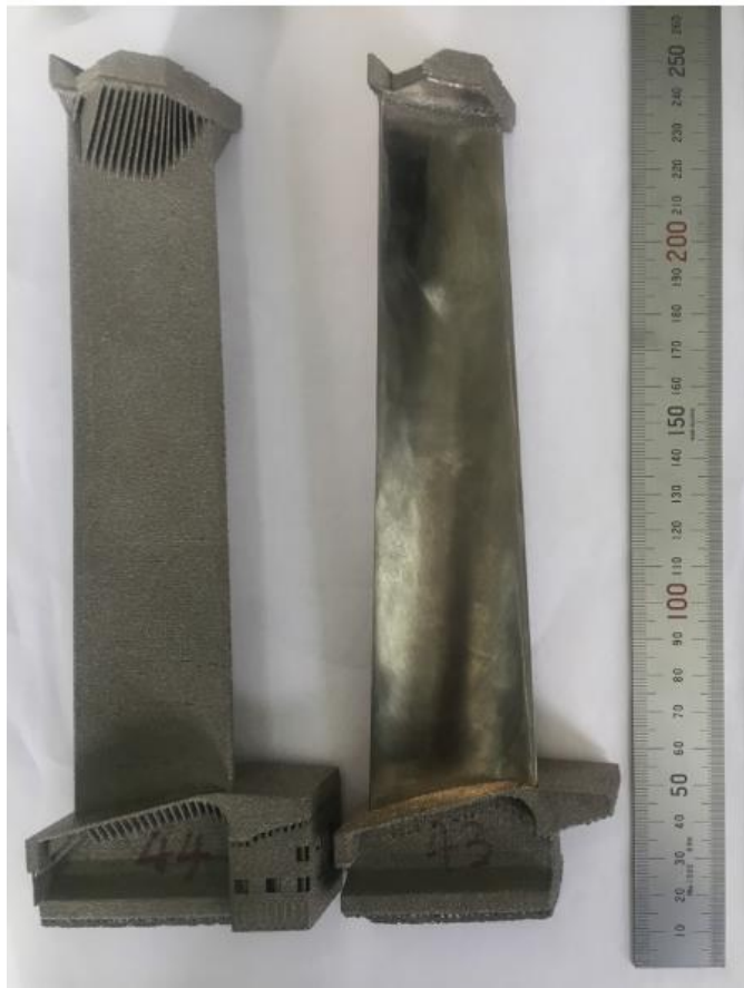
Figure 2.36: PBF-EB manufactured as-built (left) and subsequently machined (right) Ti48Al2Cr2Nb LPT blade [40].
