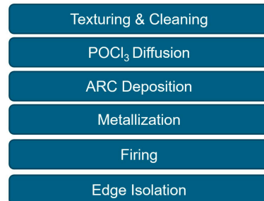
Figure 14. Process flow of Al-BSF cell production.
