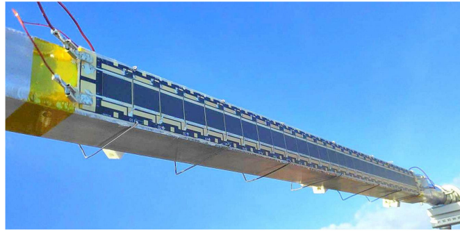
Figure 32. Photo of the CAM module installed in the parabolic trough collector for the first outdoor test operation.
