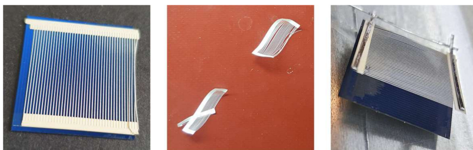
Figure 28. Detachment of electroplated silver fingers and busbars.
