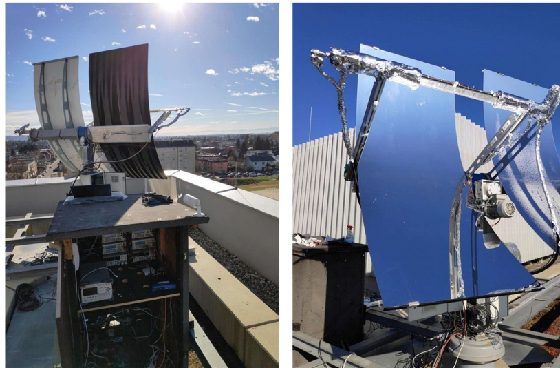
Figure 33. Final test setup in Graz, Austria. The CAM is mounted in the parabolic trough collector. The electrical measurement and control system is located in a shelter ( left ). Parabolic mirror clamped onto the injection-molded support structure capable to follow the sun by two-axis tracking ( right ).
