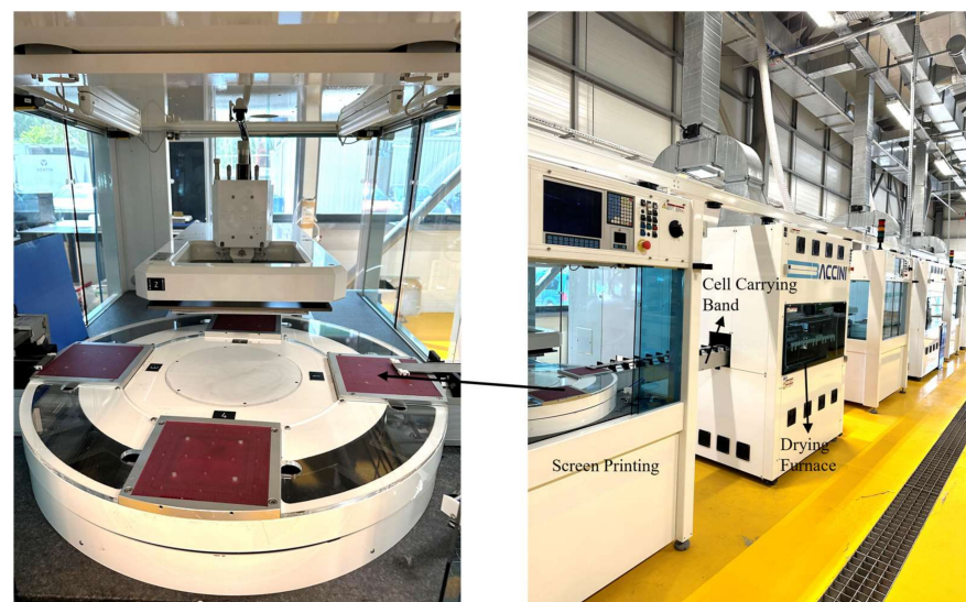
Figure 15. Solar cell metallization process.
