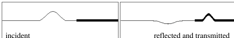
Figure 2.7. At a discontinuity (from high speed to low speed), the reflected wave changes its polarity and decreases its amplitude (Russell, 2013)
