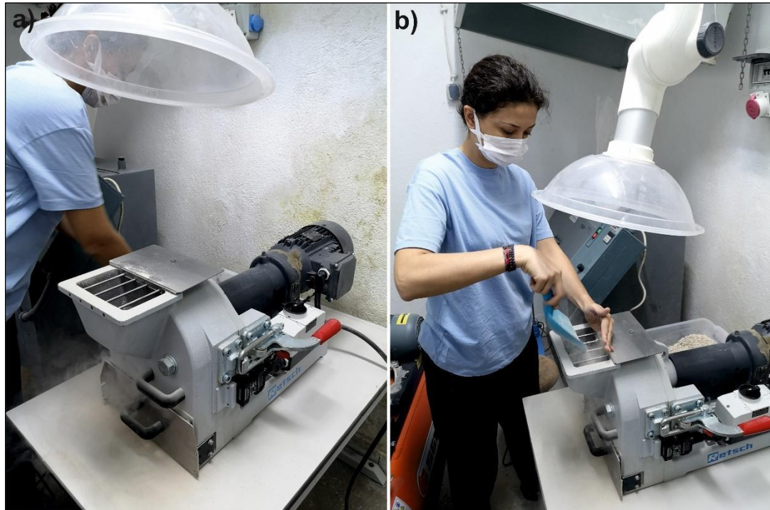
Figure 1.3. Operations with the grinder a) shows the grinder device, and b) samples from the jaw crusher are placed in the upper chamber of the grinder.
