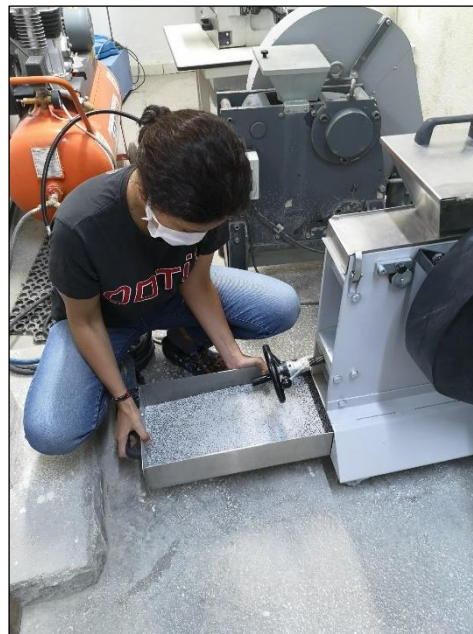
Figure 1.2. The first step of sample preparation is completed by removing the samples placed in the jaw crusher from the hopper at the bottom.
