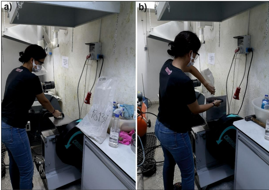
Figure 1.1. The jaw crusher is the first step in preparing samples for geochemical analysis. a) The jaw crusher is cleaned with alcohol to prevent contamination and made ready for use; b) Samples are placed in the hopper on the jaw crusher.
