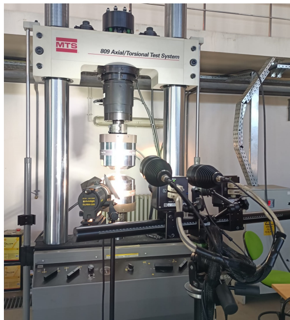
Figure 3.5: Experimental setup: Uniaxial tension test system and optical equipment for DIC measurement.
