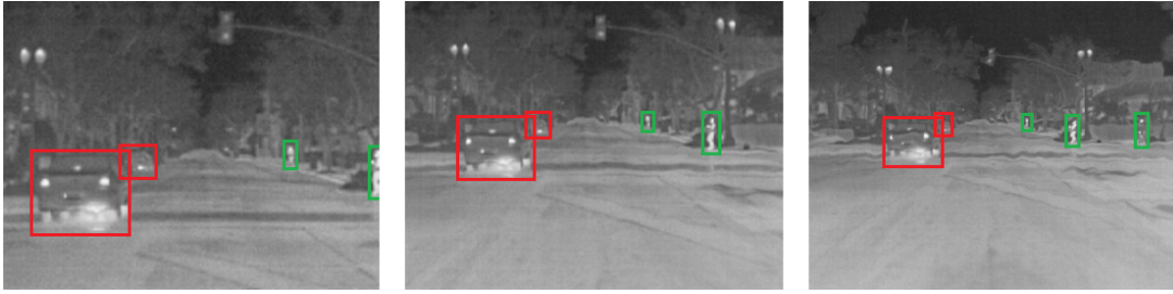
Figure 4: The leftmost image represents a patch from a sample image of the FLIR ADAS v2 dataset. The middle and rightmost images are patches from the same image, created using the proposed geometric turbulence model with \gamma values of 50 and 100, respectively. Annotations for the person and car classes are indicated by colored rectangles.
