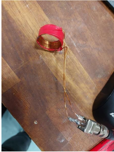
Figure 2.5 The solenoid coil build for the system
