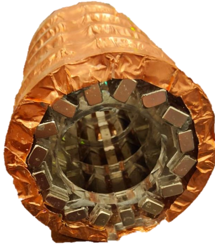
Figure 2.4 Cropped Photograph of Crafted NMR Probe with covered with copper foil
