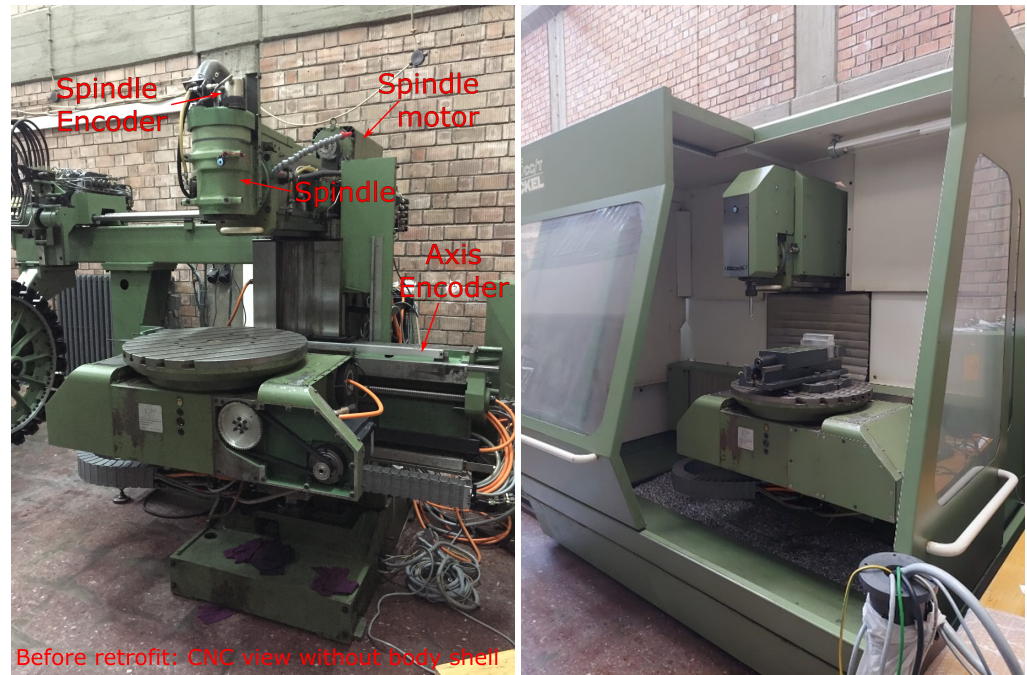
Figure 4. The in-house retrofitted Deckel FP5cc/T CNC; a PC-based controller with TwinCAT software allows the implementation of ACC algorithm together with the CNC-related motion control tasks.
