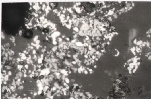
Figure 22e. Microphotograph of Pellet of Hekimhan Sideritic Iron Ore Fine Indurated at 1200°C and Suddenly Cooled in Air (400 X),
