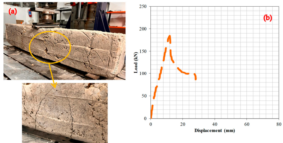
Figure 8. RCBs under perpendicular loads, (a) cracking and bending behaviors, (b) load–deformation attitudes of RCBs with 30% WAD.
