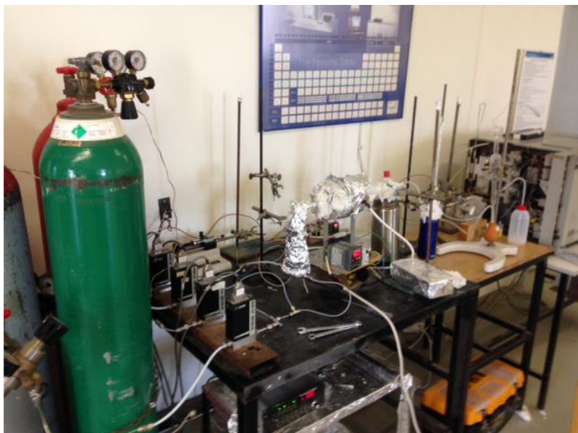
Figure 1. The fixed-bed reaction setup used for dry reforming experiments.
