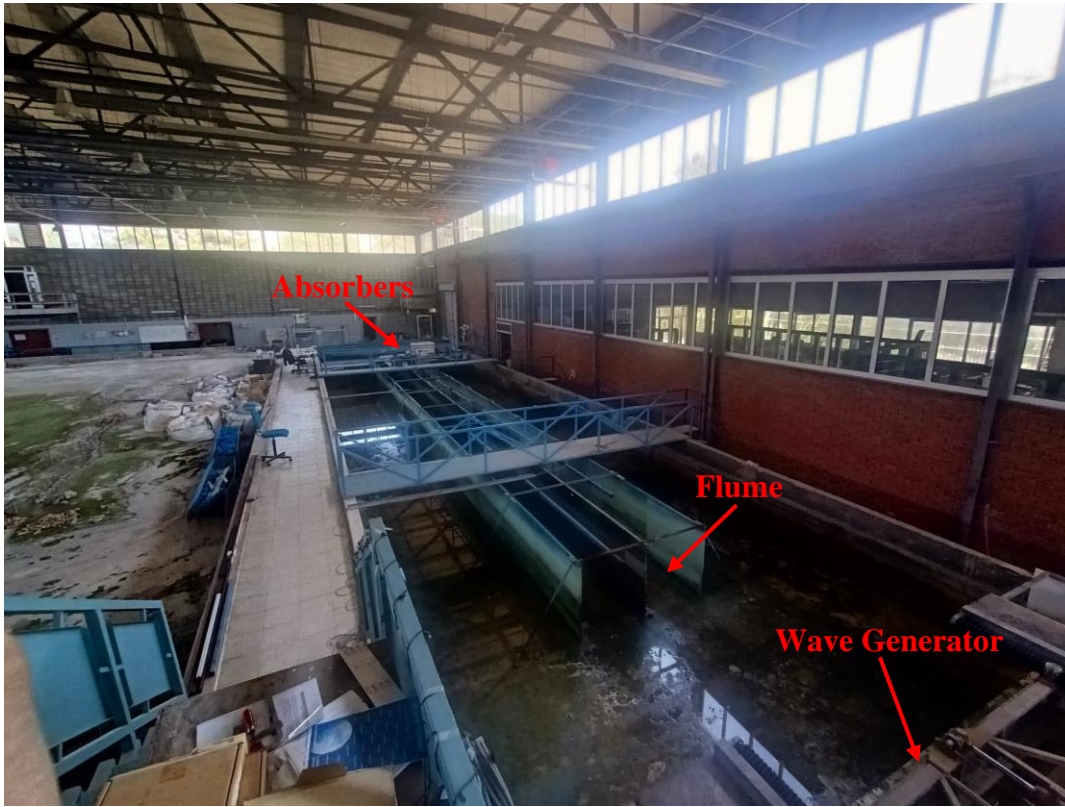
Figure 3.1. General view of the wave flume at Middle East Technical University.
