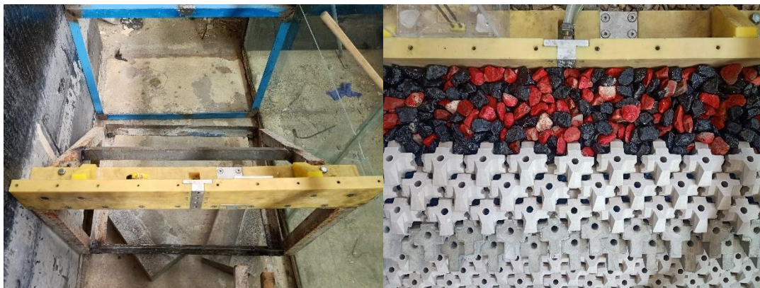
Figure 3.6. Crown wall model
