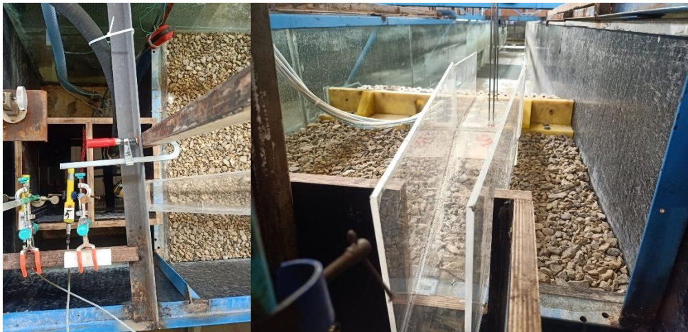
Figure 3.8. The collecting system for wave overtopping
