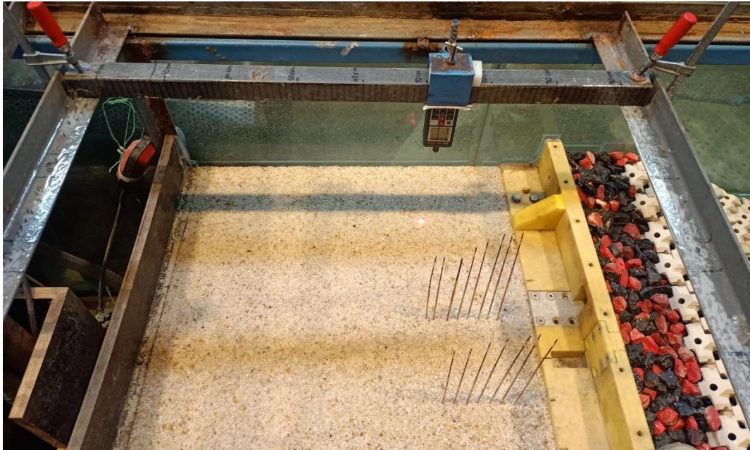
Figure 3.11. Profile measurement setup
