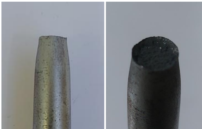
Figure 5.8: Side and Top Views of Fracture Surface at Fatigue Test 4
