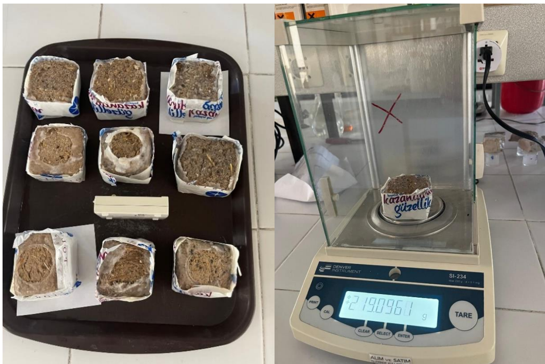
Figure 3-13. (Left) Samples left to dry and weighed periodically to calculate their Drying Index (Right) weighing samples during the drying phase.
