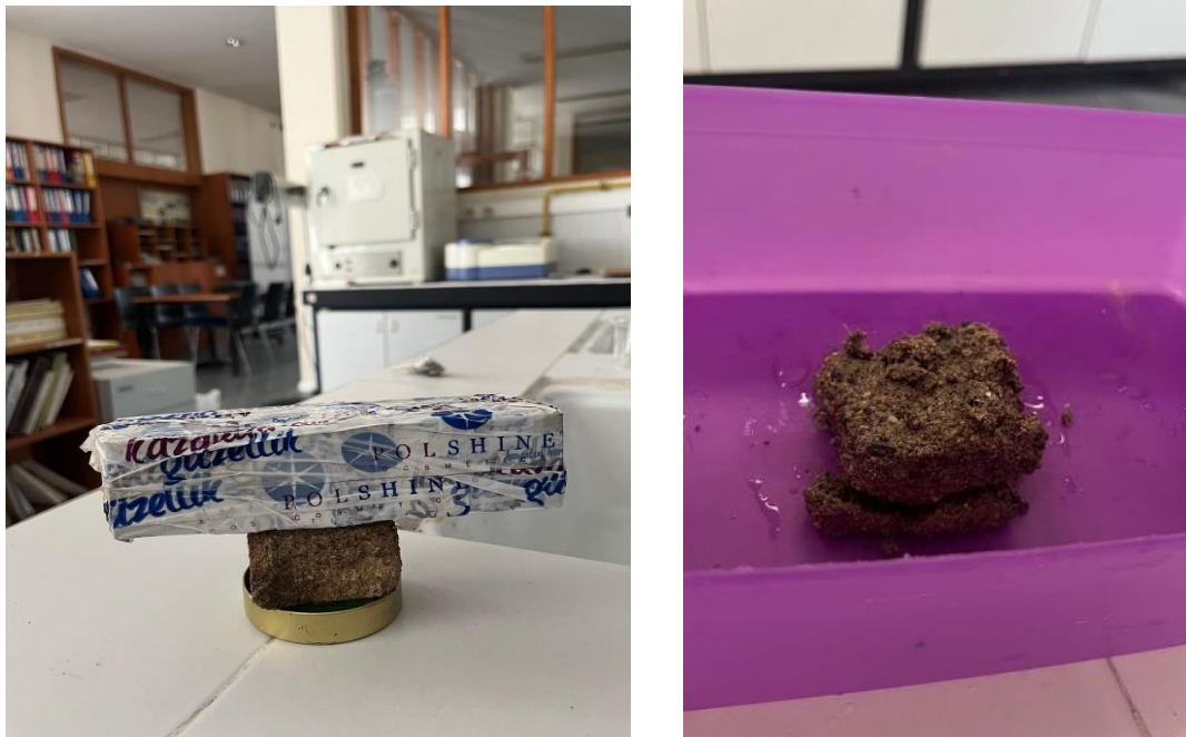
Figure 3-8. (Left) Sample under the 3kg weight with wet sponge (Right) result of Result of absorption on the test sample.
