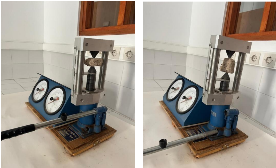
Figure 3-6. (Left) Horizontal sample placement (Right) Vertical sample placement.
