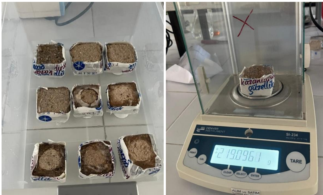
Figure 3-12. (Left) Water capillary absorption test setup (Right) weighing absorbed water content.
