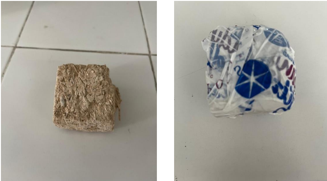
Figure 3-4. (Left) Samples without any covering (Right) wrapped sample for Archimedes experiment.
