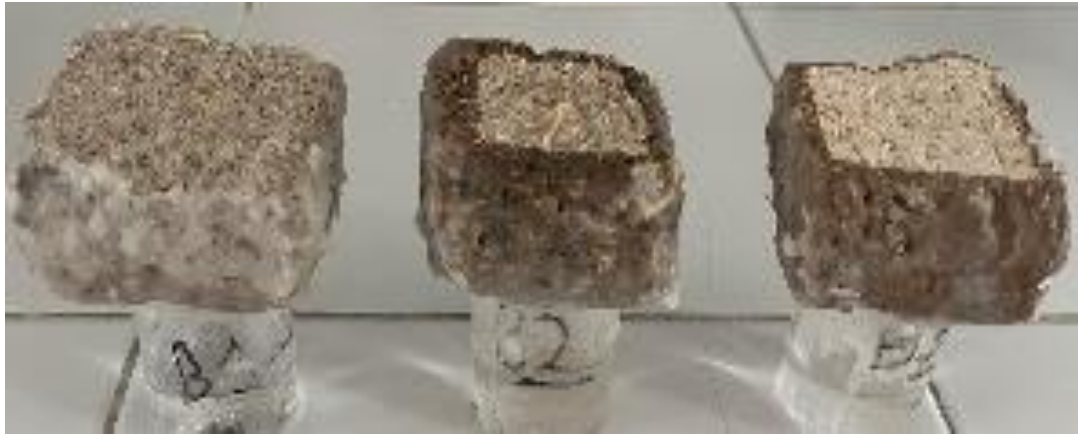
Figure 3-14. Wet cup water vapour permeability test showing samples B1, B2 and B3
