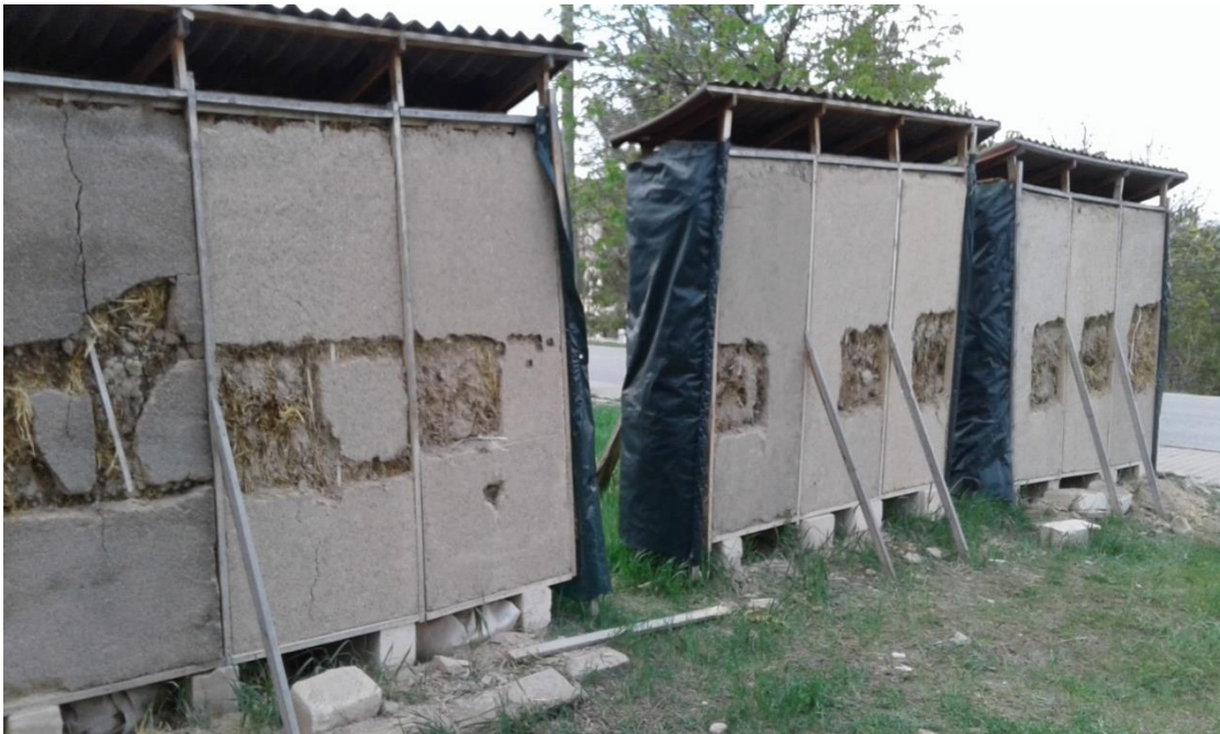
Figure 3-2. Strawbale wall samples removed from the 9 panels A1(KeSdMo), A2 (KeSdFbEg), A3 (KeSdFbCd), B1 (KeSd), B2 (KeSdFb-1), B3 (KeFb), C1 (KeSdFbDj), C2 (KeFbCd), C3 (KeSdFb-2) (ordered left to right)
