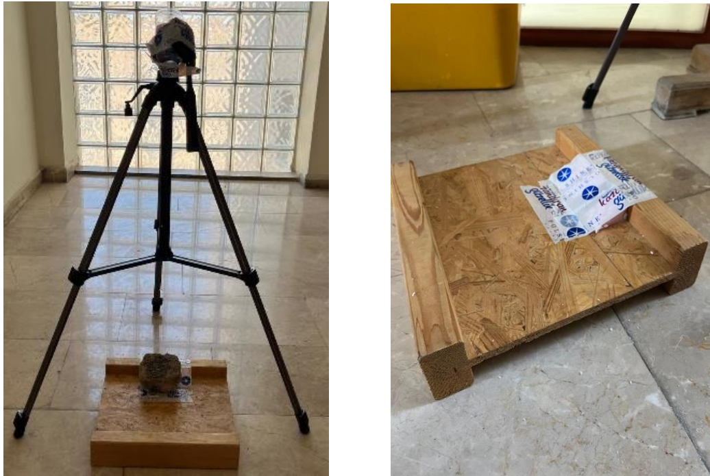
Figure 3-10. (Left) Erosion test setup (Right) 30° sloped sample's base for erosion test.
