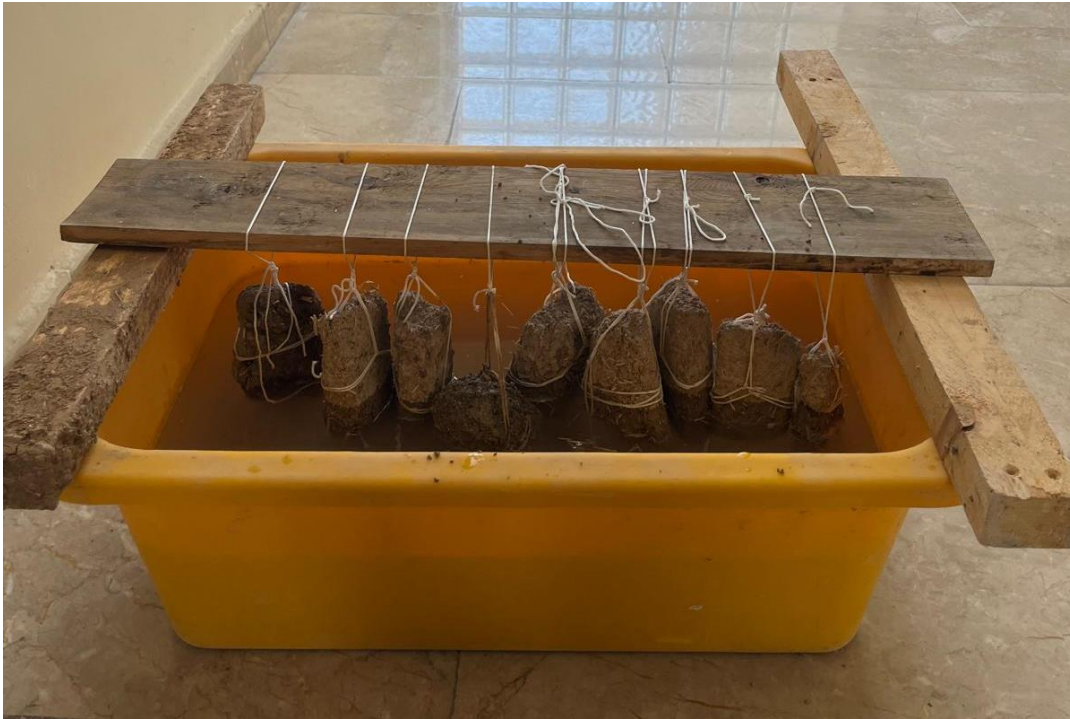
Figure 3-9. Water resistance test, A1(KeSdMo), A2 (KeSdFbEg), A3 (KeSdFbCd), B1 (KeSd), B2 (KeSdFb-1), B3 (KeFb), C1 (KeSdFbDj), C2 (KeFbCd) and C3 (KeSdFb-2), ordered left to right.
