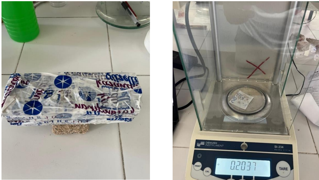
Figure 3-7. (Left) Sample under the 3kg weight (Right) Adhesive tape with stuck material.
