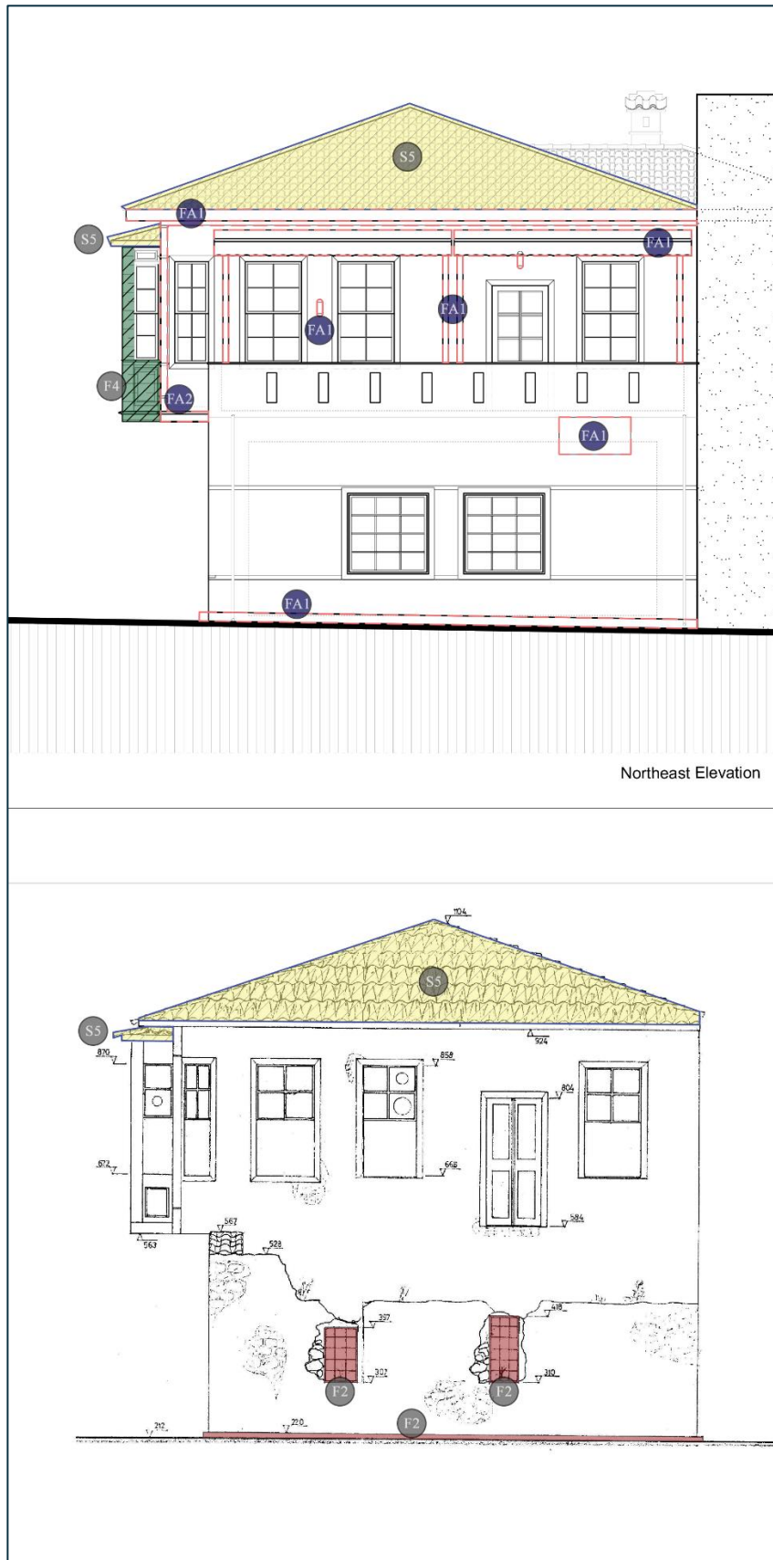
Figure 4.9. Restored (up) and original northeast elevation value shift analysis. Prepared by the Author.
