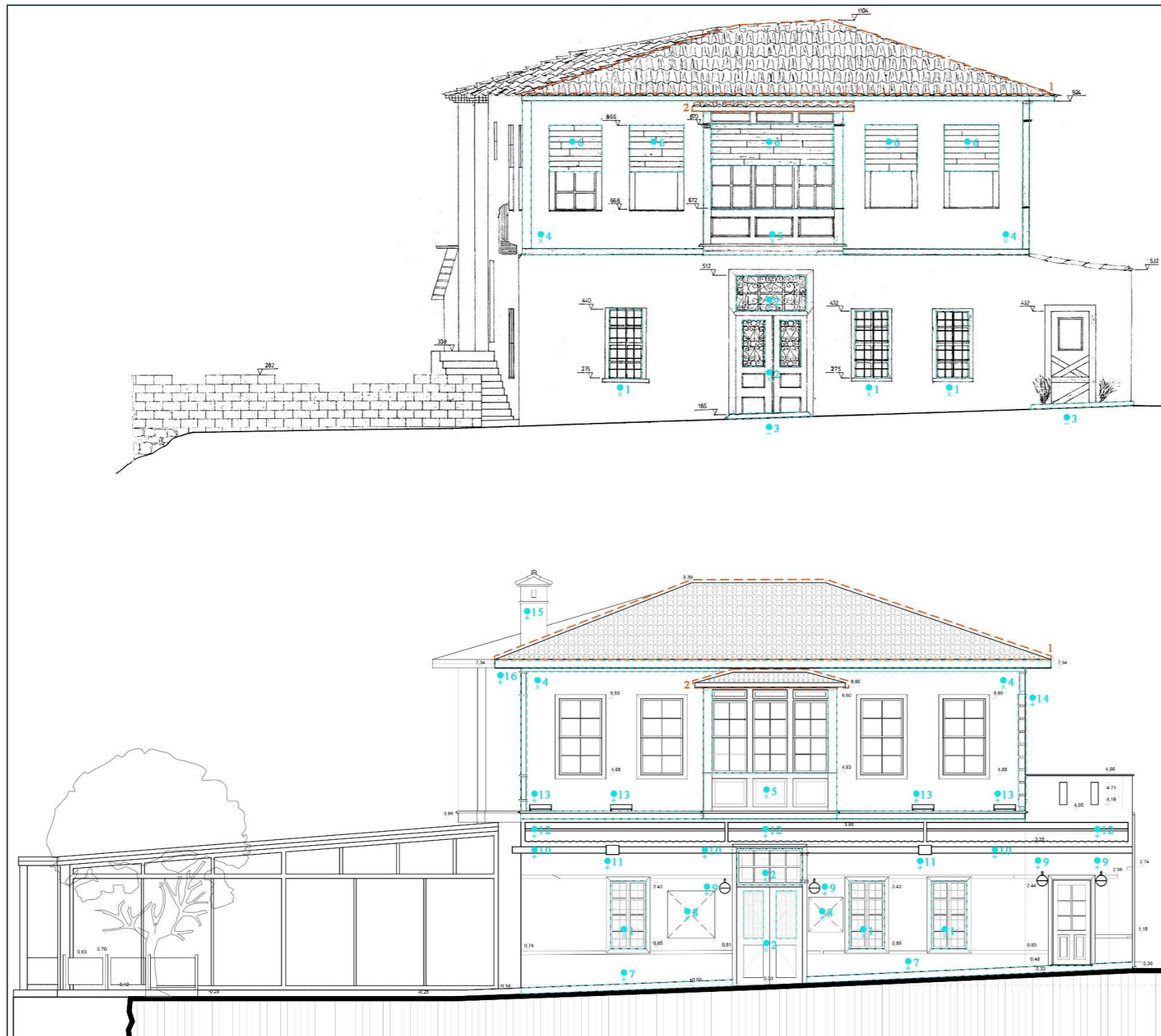
Figure 3.55. Restored (bottom) and original (top) southeast elevation intervention analysis of Building A. Prepared by the Author based on the official original and restoration drawings.
