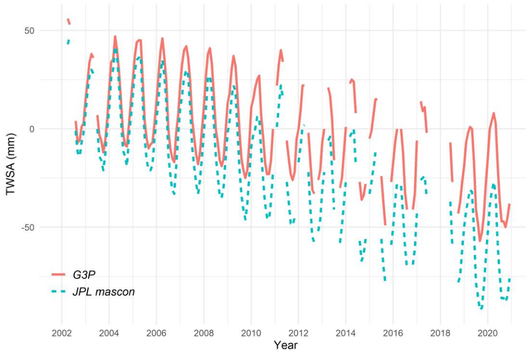
Figure 2.5. The time series of the global mean monthly TWSA dataset obtained from G3P and JPL
