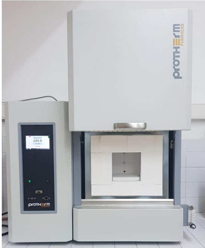
Figure 3.5 The chamber furnace used for the heat treatments.
