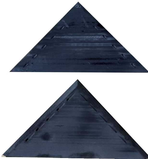
Figure A.5: Nozzle bleed wing narrow CR050 rear ( \Lambda = 45^\circ , t/c = 5.9\% ).
