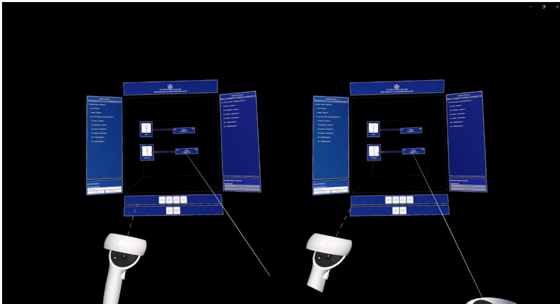
Figure 33 – Visualization of use case diagram in MRSysML designed by the user with controller interaction method with view from both eyes.
