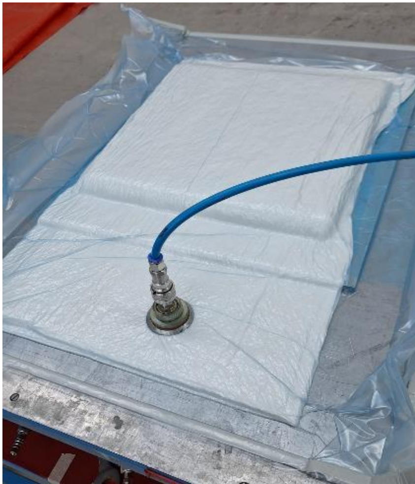
Figure 3.7 Vacuum bagging of the polybenzoxazine composite
