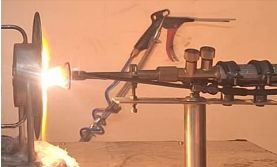
Figure 4.13 Oxyacetylene test equipment during ablation testing
