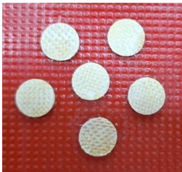
Figure 3.11 Thermal diffusivity test samples of polybenzoxazine composites
