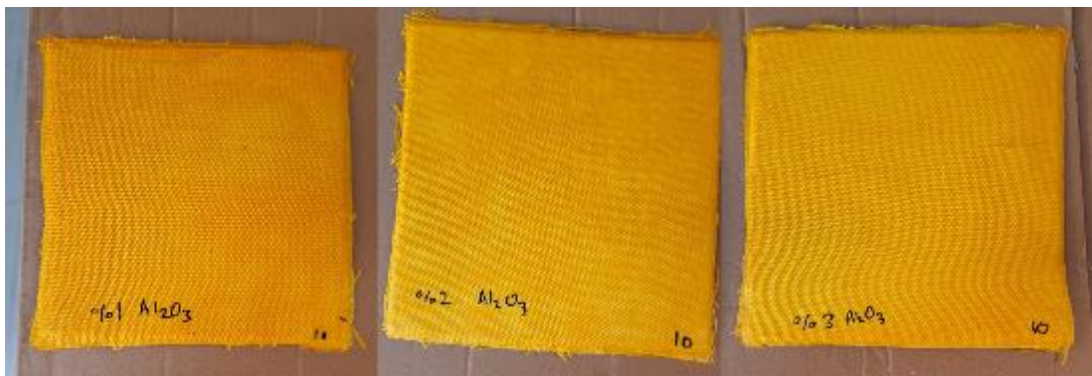
Figure 3.9 Finished Polybenzoxazine composites reinforced with alumina particles
