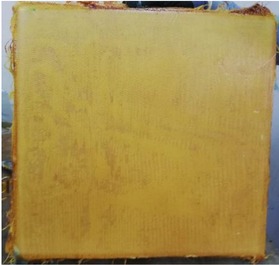
Figure 3.8 Neat polybenzoxazine composite after curing in autoclave
