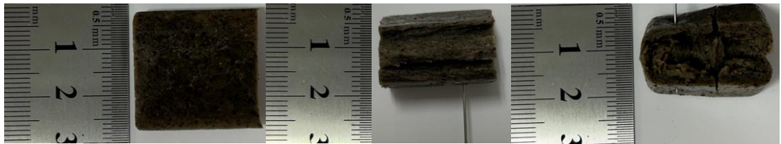
Figure 20: HMMA, H:SPI_50:50, 65% moisture, 125°C. Images of surface, longitudinal to flow and transversal to flow, respectively
