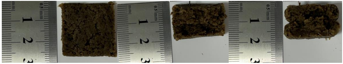
Figure 12: HMMA, H:SPI_50:50, 65% moisture, 100°C. Images of surface, longitudinal to flow and transversal to flow, respectively
