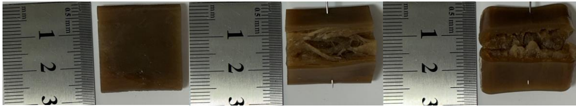
Figure 15: HMMA, H:SPI_0:100, 65% moisture, 125°C. Images of surface, longitudinal to flow and transversal to flow, respectively
