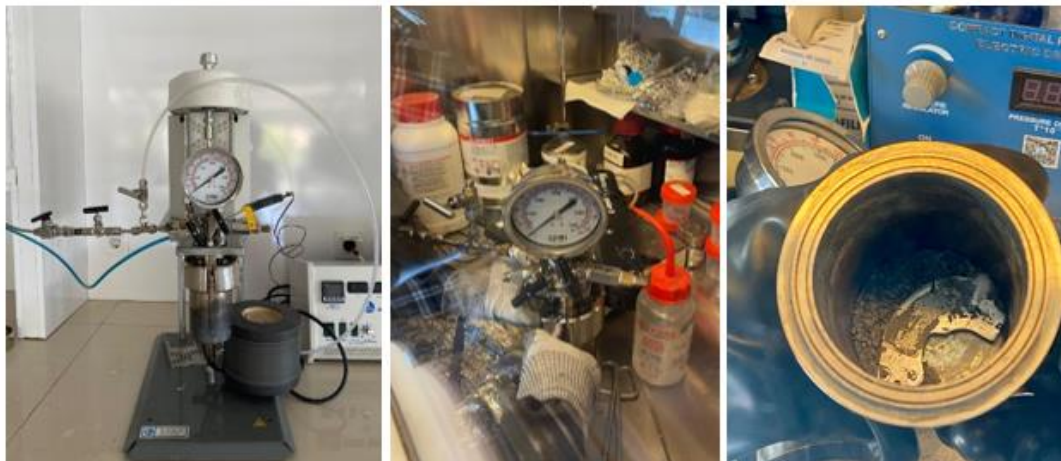
Figure 3.4 a) The hydrogenation reactor b) Preparation of the reactor in the glove box c) Magnet powders separated from the VCM assembly after the HD process
