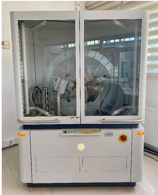
Figure 3.10 X-ray diffractometer (Malvern Panalytical/Empyrean).
