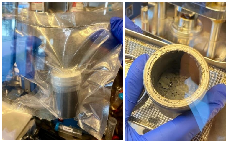
Figure 3.6 a) Placement of the jar in a vacuum pack to prevent oxygen contact during the BM process b) Dried powders after the BM process
