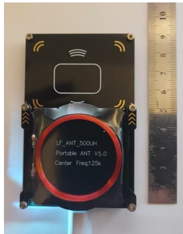
Figure 3: Proxmark3 Hardware with Low Frequency and High Frequency Antenna
