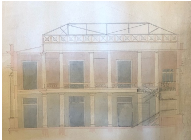
Figure 269. The original drawing of Vallaury period showing the roof structural system (source: “IAM Archive, 16-G2/R2/3”)
