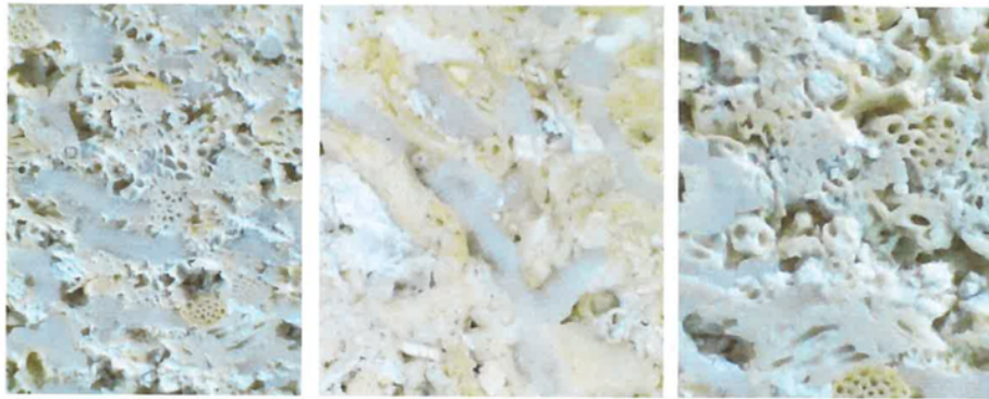
Figure 172. Micro Capture USB Microscope Viewed from cross-sectional surface. There is plenty of bryazone, diatomite and a few nummulites. (source: 26.01.2012 dated Istanbul Restoration and Conservation Regional and Central Laboratory Directorate Report prepared by İsmet OK, IDSMS Archive)
