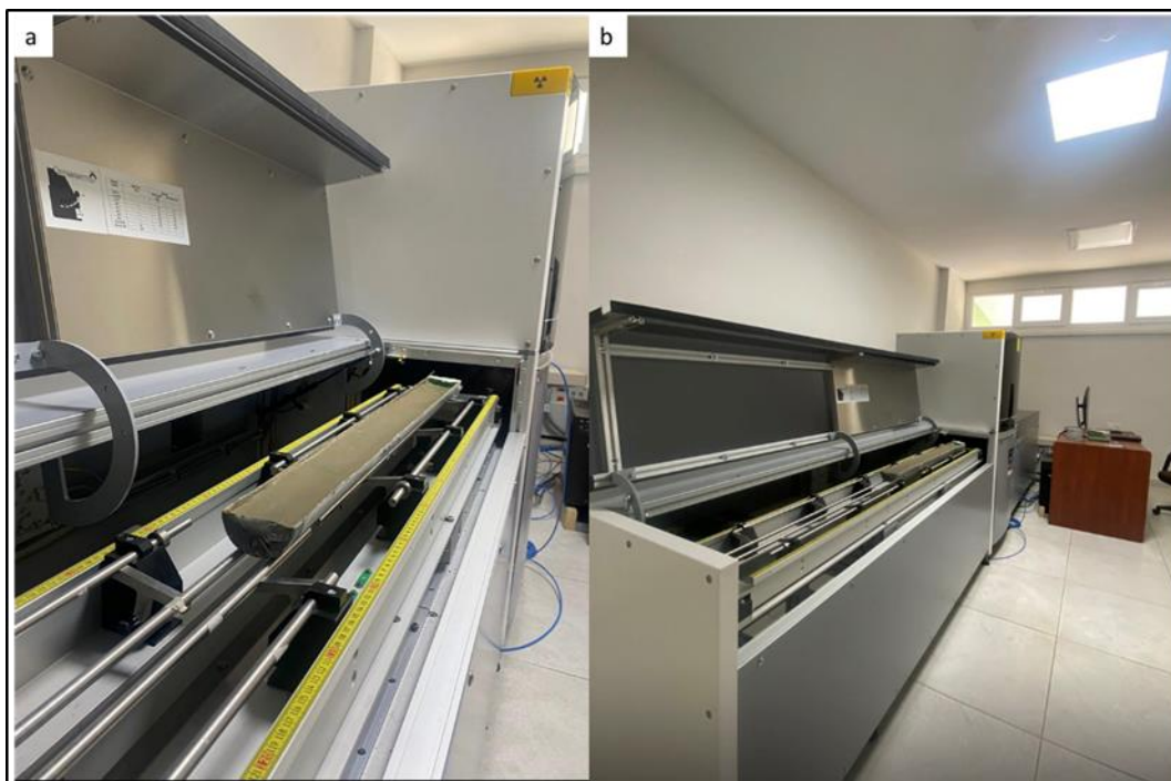
Figure 3.7 (a) Core sample and (b) ITRAX \mu XRF core scanner
