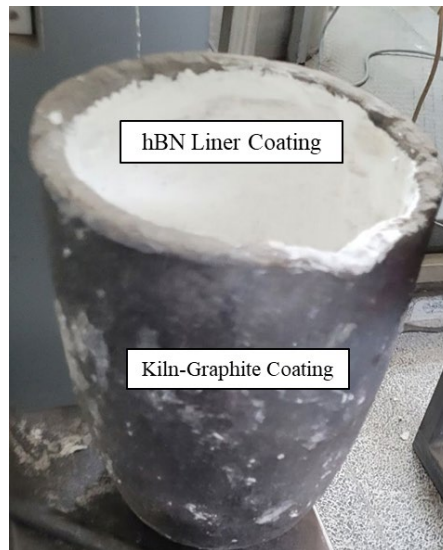
Figure 3.2. Kiln-Graphite crucible, where the inner wall is coated with hBN and serves as a liner.
