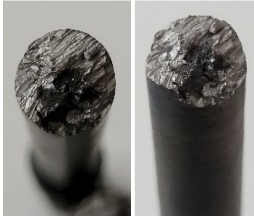
Figure 4.8. Sample 1 fracture surface after tensile test.
