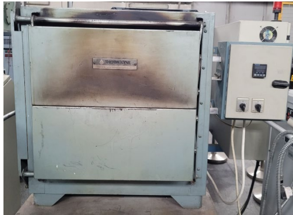
Figure 3.7. Box furnace used for homogenization, solutionizing, and aging heat treatments.
