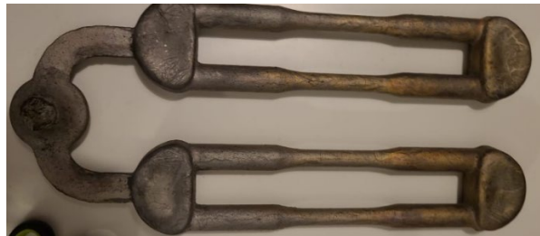
Figure 4.4. Sand casting product with runners and risers attached.
