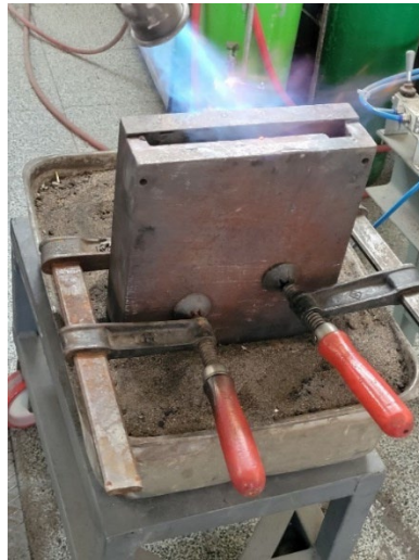
Figure 3.5 Metal mould is held by two holders. A flame is heating up to metal from the above.
