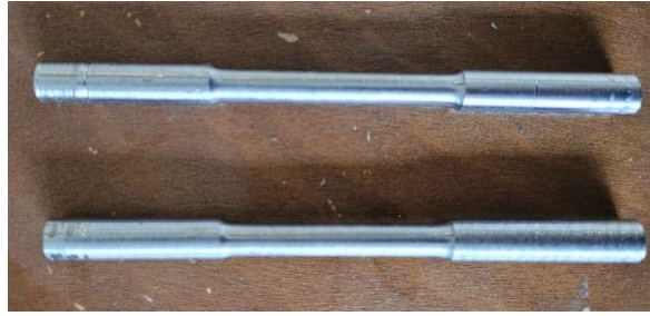
Figure 4.6. Tensile specimens from metal mould castings after machining.
